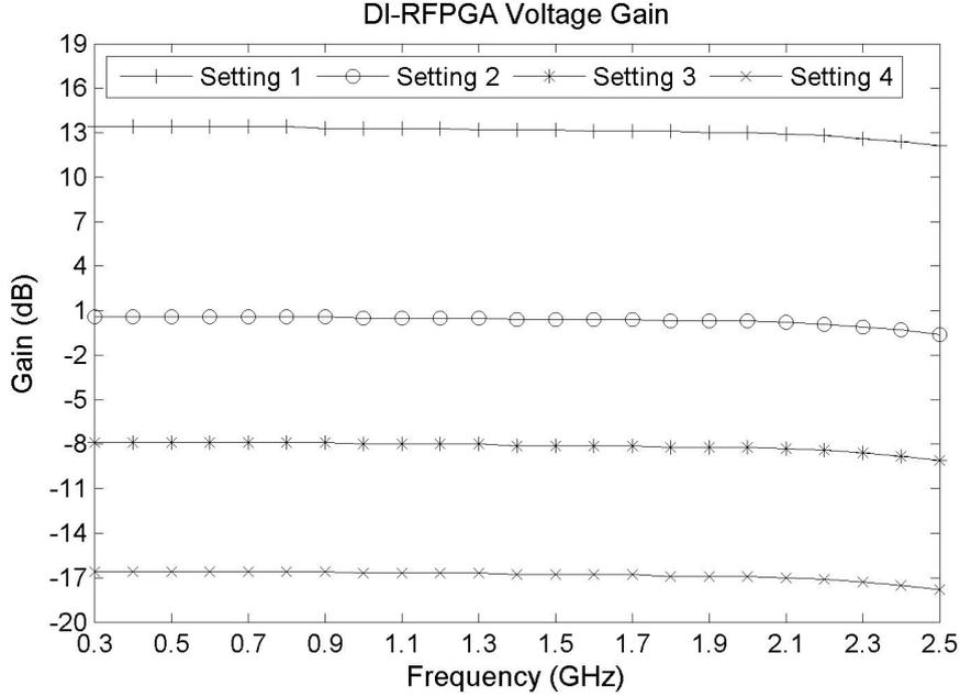
**Figure 5.12:** DI-RFPGA voltage gain measurement results.
