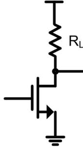
**Figure 3.11:** Basic topology of an amplifier with resistive load.
