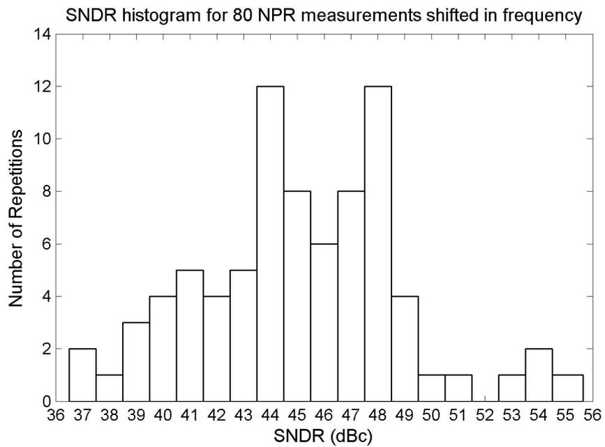
**Figure 6.19:** Histogram of the NPR notch measurements.
