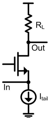
**Figure 3.5:** Basic topology of the common-gate input impedance matching.
