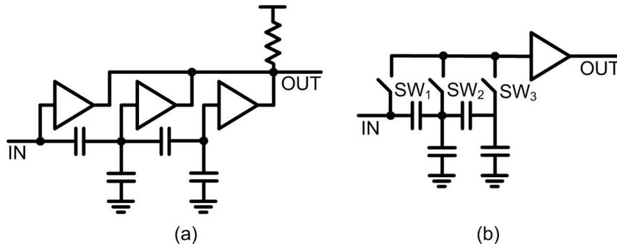
**Figure 4.1:** Capacitive attenuation topology, (a) Nonswitchable (b) Switchable
