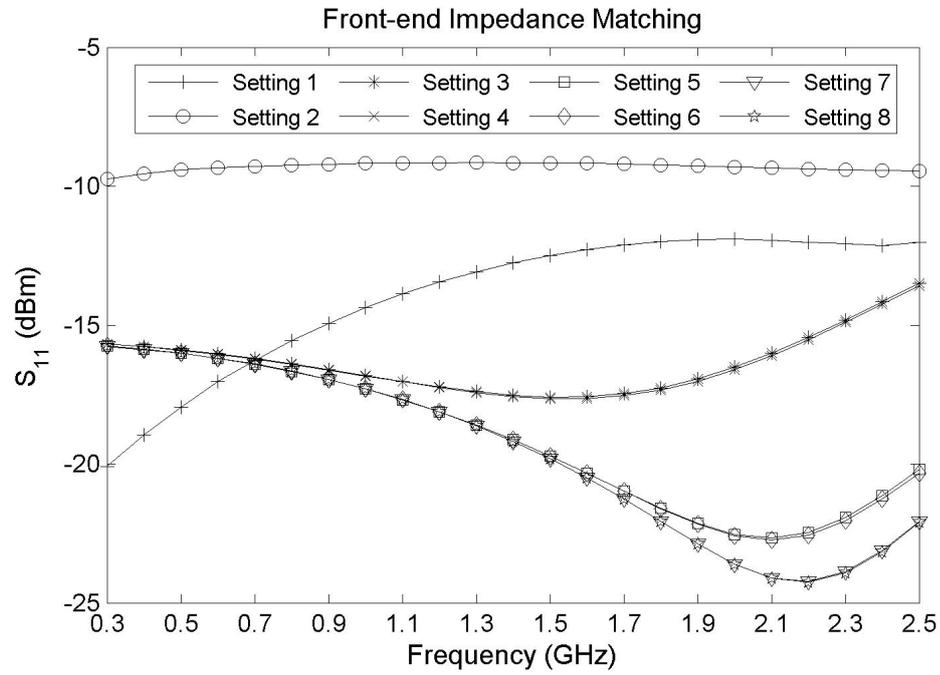
Figure 6.10: Front-end  $s_{11}$  measurement results.
