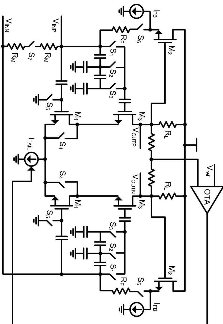
Figure 5.2: Schematic of the differential double-input RFPGA with switchable capacitive attenuation.
