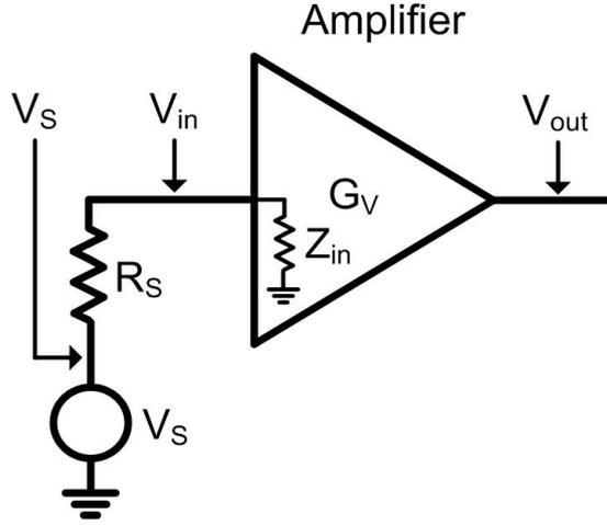
Figure 4.10: Input structure of a front-end.
