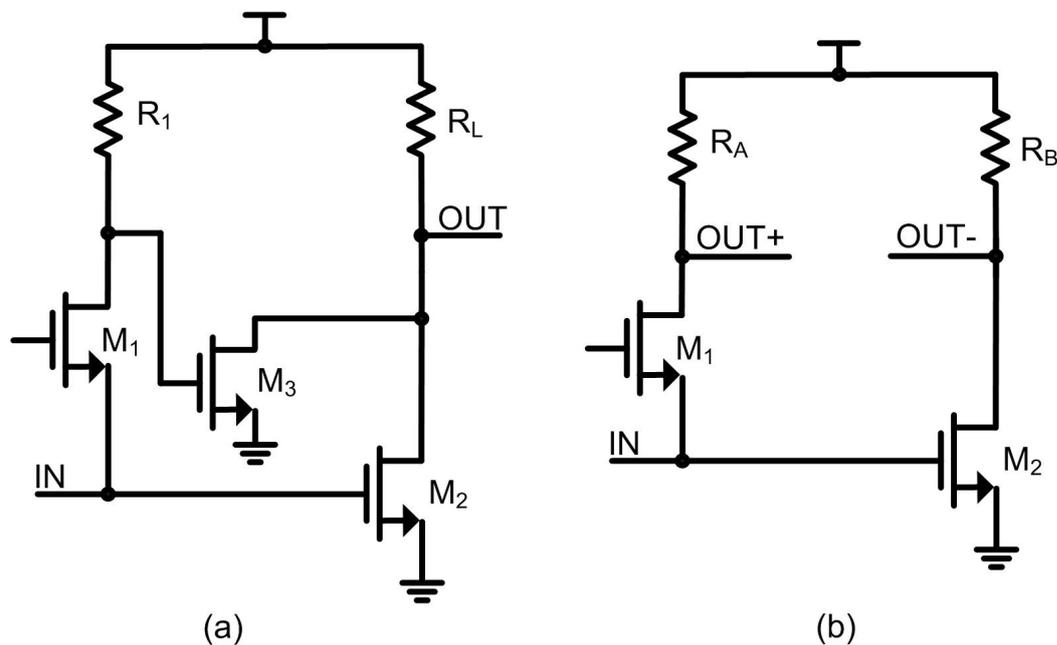
**Figure 3.20:** Noise/distortion cancellation topologies (a) Single-ended (b) Single-ended to differential conversion.
