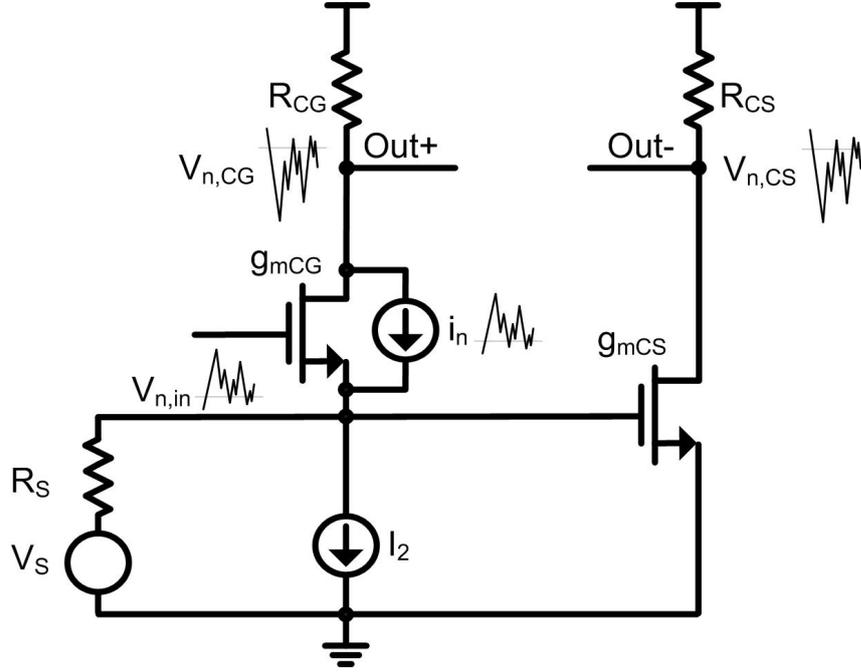
**Figure 3.8:** Combined common-gate common-source topology providing simultaneous input impedance matching, single-ended to differential conversion and noise-canceling.
