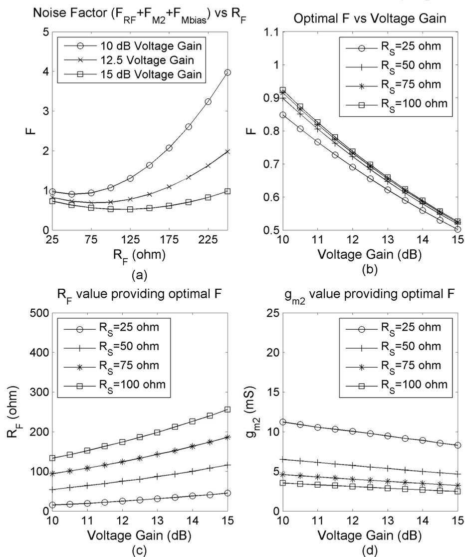
**Figure 4.8:** Optimization of the noise generated by  $R_F$ ,  $M_2$  and  $M_{bias}$ ; (a) Noise factor dependency on  $R_F$  and  $A_v$  (b) Optimal noise factor for different values of  $A_v$  and  $R_S$  (c)  $R_F$  resistance value that provides optimal noise factor for different values of  $A_v$  and  $R_S$  (d)  $M_2$  transconductance value that provides optimal noise factor for different values of  $A_v$  and  $R_S$ .
