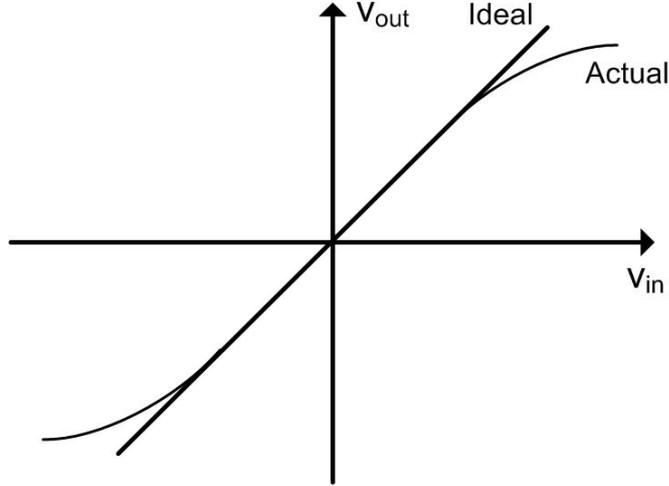
**Figure 2.1:** Actual versus ideal behavior of an amplifying device.
