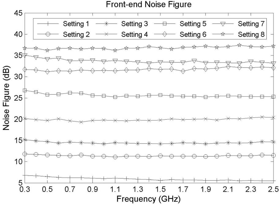
**Figure 6.12:** Front-end noise figure measurement results.
