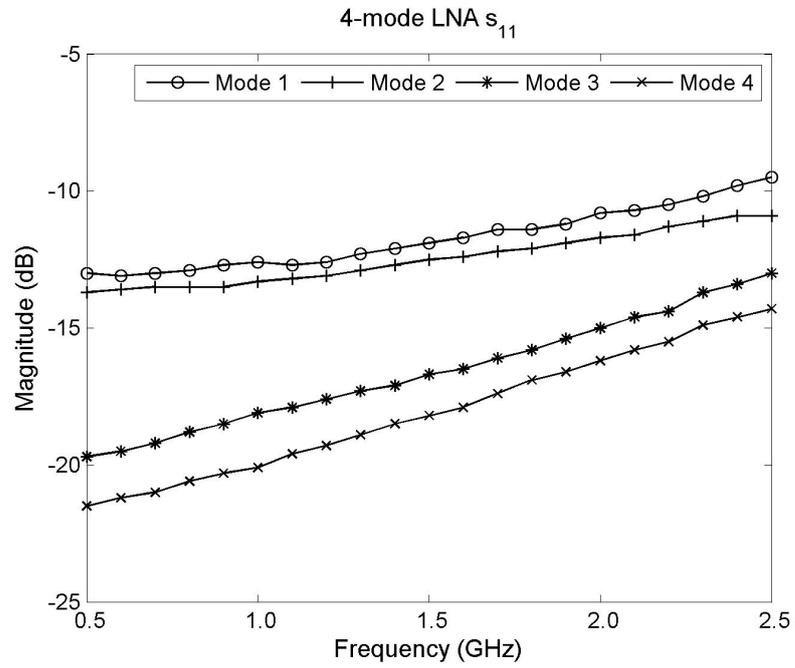
Figure 4.16: Measured  $s_{11}$  of the RFPGA four settings.
