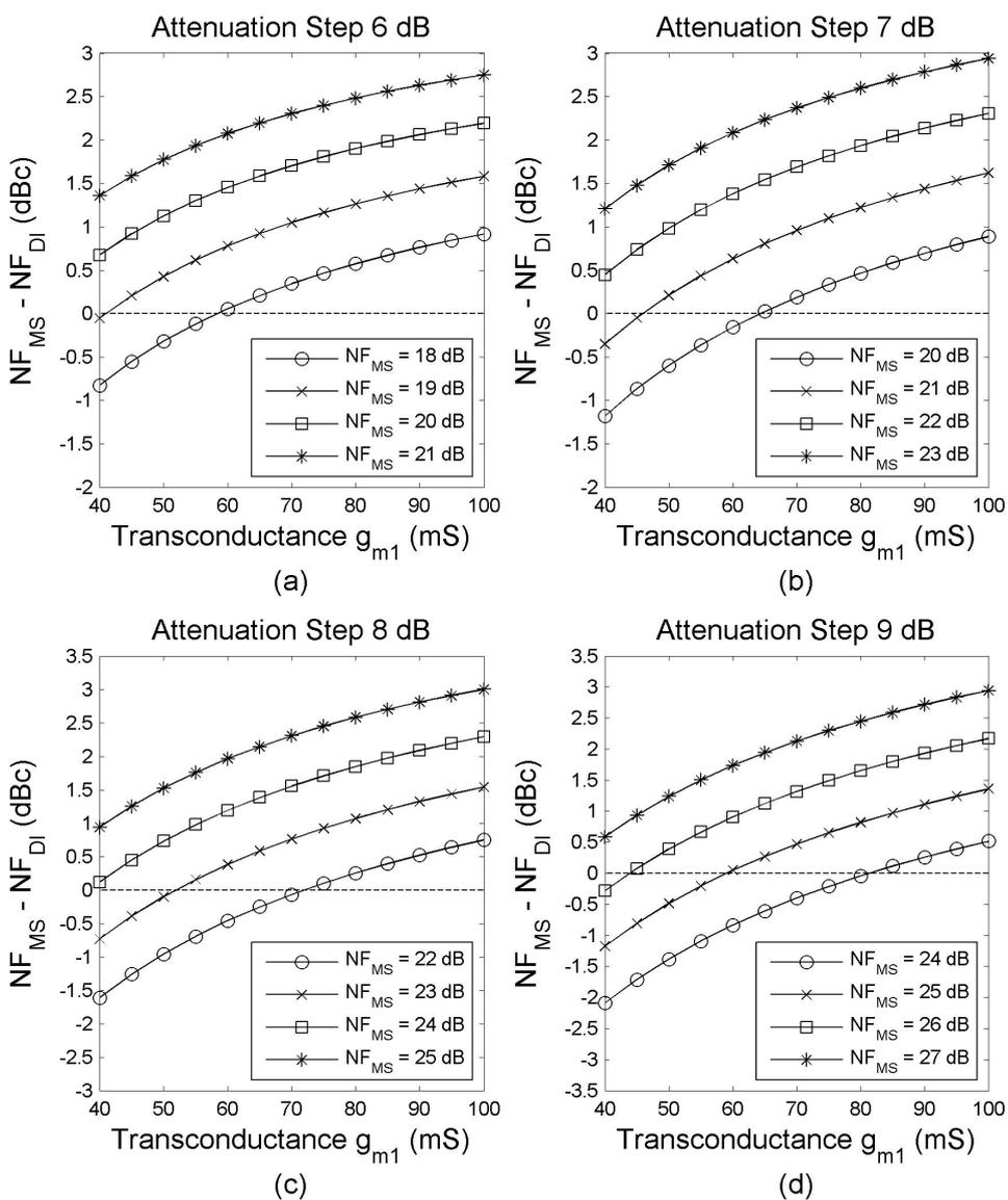
**Figure 5.11:** Noise figure difference between the MS and the DI topologies (Gain Setting 4) for different values of transconductance, MS noise figure and attenuation step.
