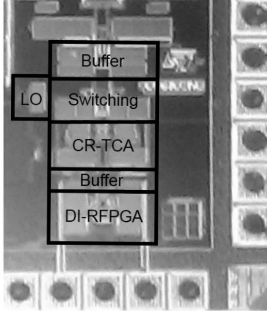
Figure 6.8: Front-end prototype microphotograph.
