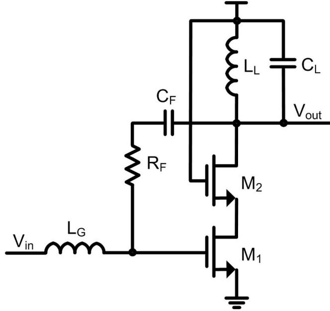
**Figure 3.3:** Resistive feedback using input inductor.
