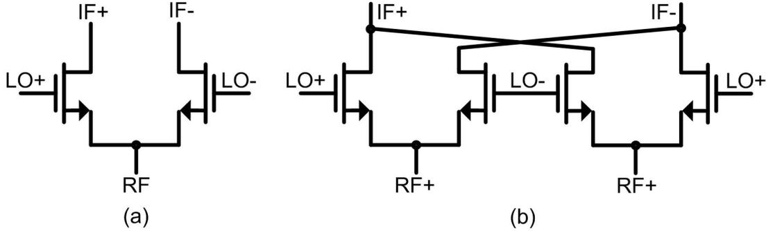
Figure 2.10: Common mixer implementation in CMOS (a) Single-ended (b) Differential.
