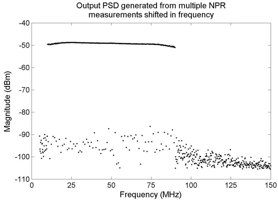
**Figure 6.18:** Full channel output spectrum containing all the individual NPR notch measurements.
