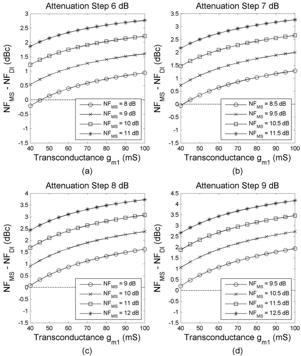
**Figure 5.9:** Noise figure difference between the MS and the DI topologies (Gain Setting 2) for different values of transconductance, MS noise figure and attenuation step.
