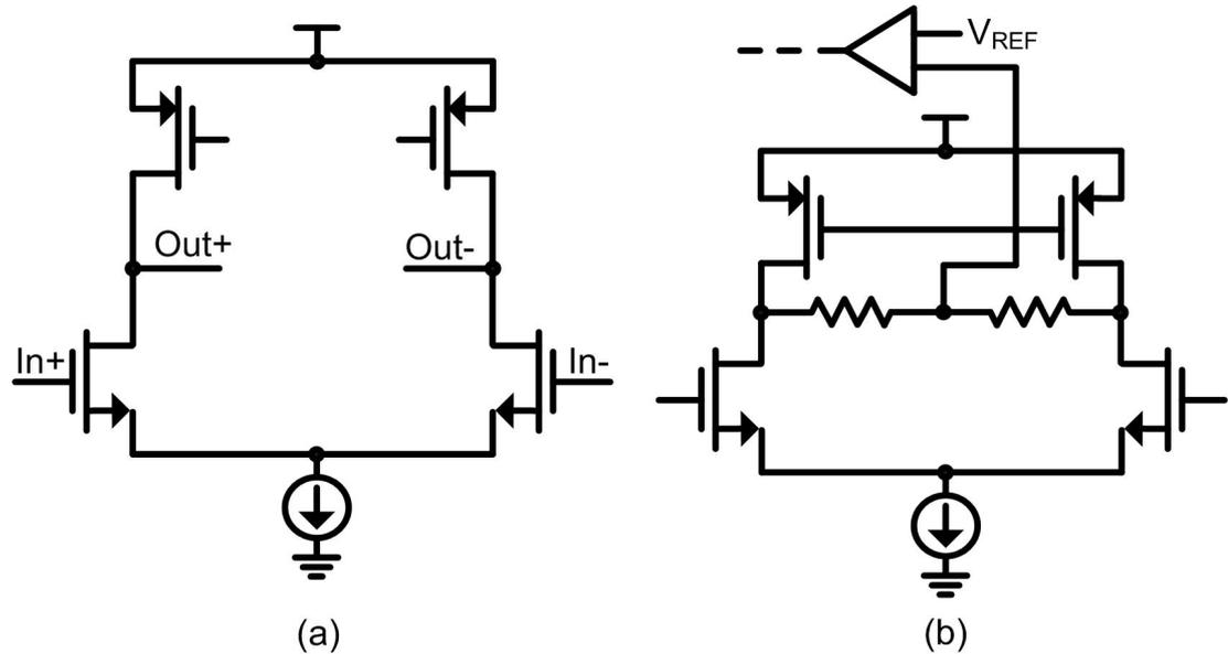
**Figure 3.12:** Basic topologies of a circuit with active loads (a) Differential amplifier with PMOS loads (b) Differential amplifier with active loads and CMFB.
