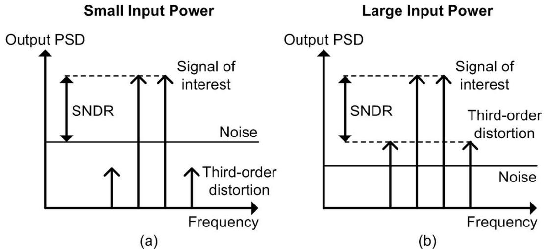
**Figure 2.4:** SNDR calculation at (a) Small input power (b) Large input power.
