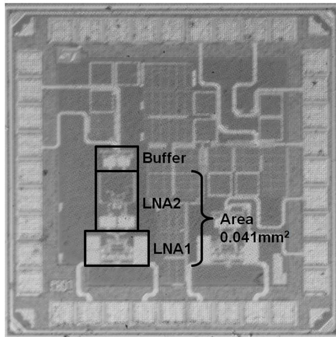
Figure 4.14: Microphotograph of the RFPGA.
