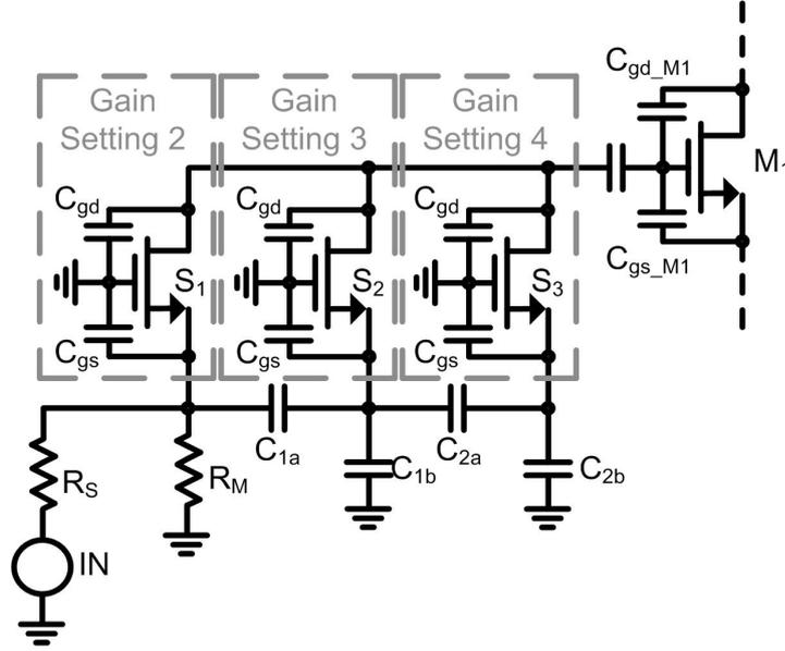
**Figure 4.5:** Capacitor ladder including the parasitic capacitances of the switches.
