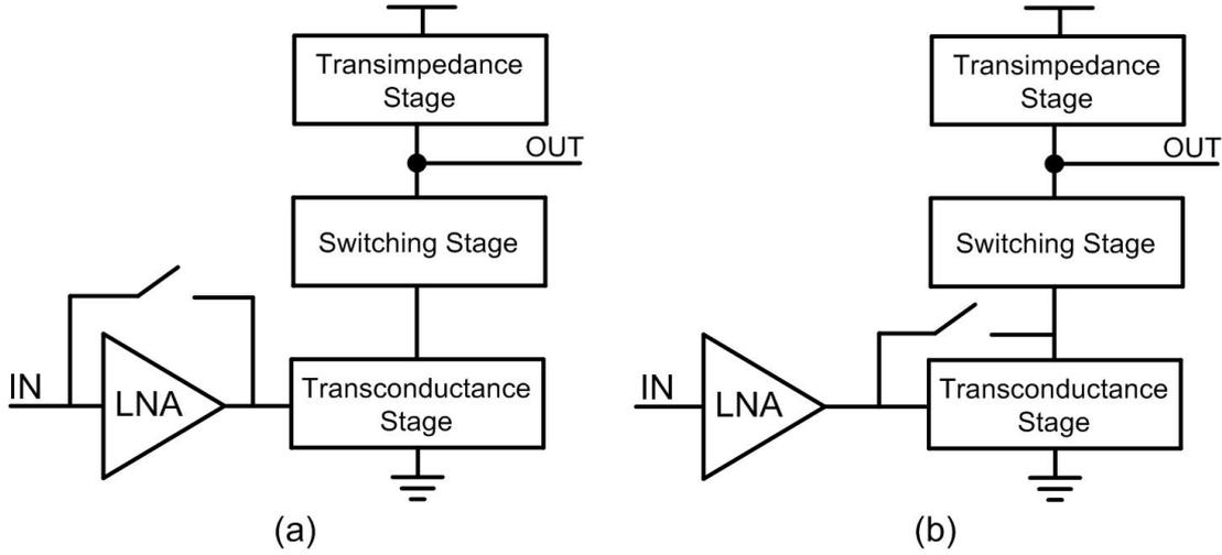
**Figure 6.2:** (a) Front-end with by-passable LNA and (b) Front-end with by-passable mixer transconductance.
