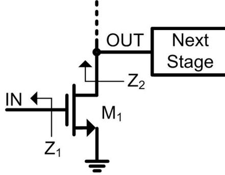
**Figure 3.19:** Impedances affecting the behavior of the harmonic termination third-order cancellation technique.
