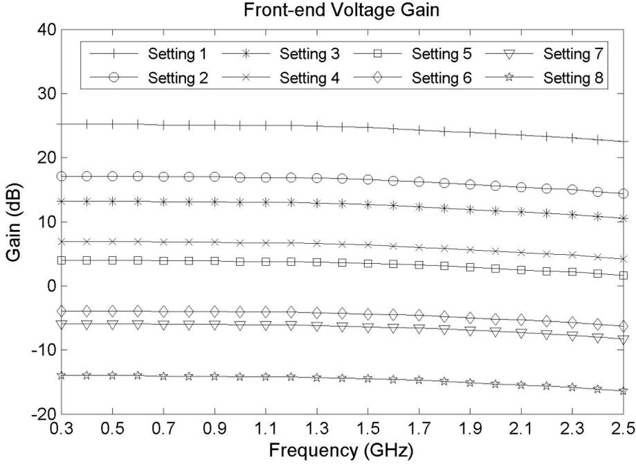
Figure 6.9: Front-end voltage gain measurement results.
