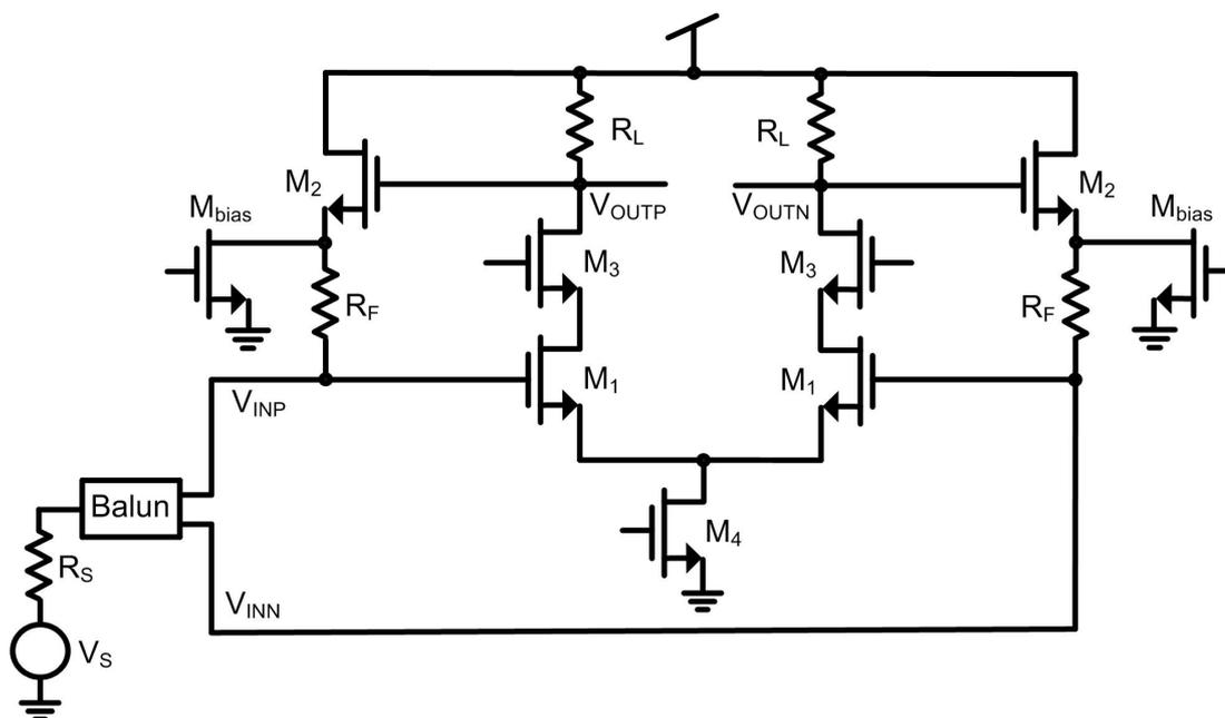
**Figure 5.7:** DI-RFPGA simplified schematic used for noise calculations at the highest-gain setting.
