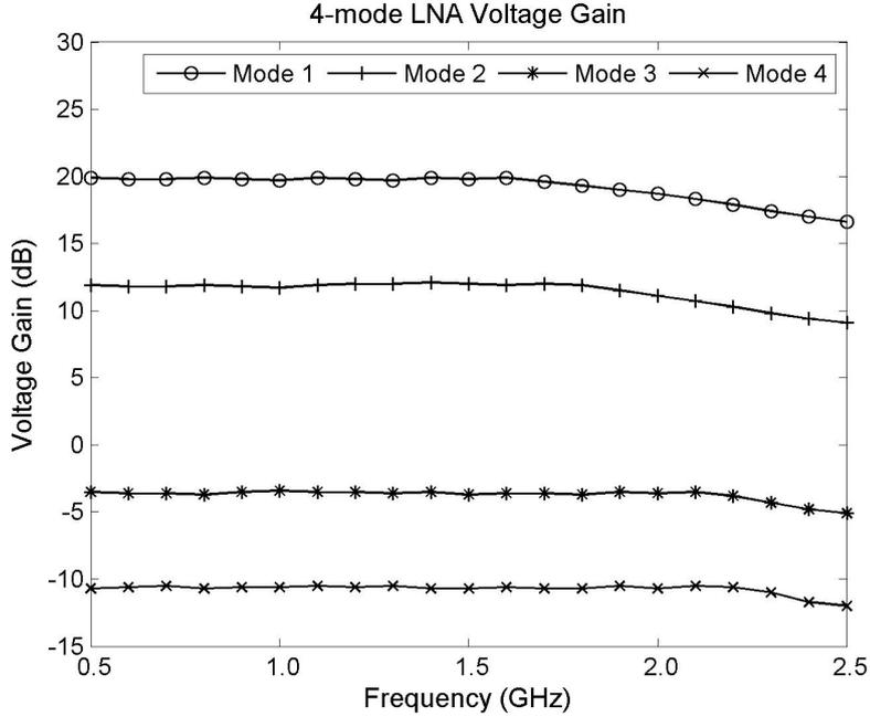
**Figure 4.15:** Measured voltage gain of the RFPGA four settings.
