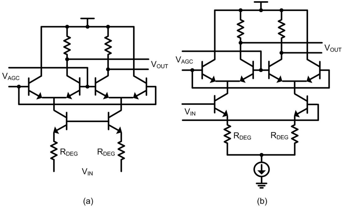
**Figure 3.25:** Variable- $G_m$  amplifiers with current steering and degeneration: (a) Common-gate (b) Common-source.
