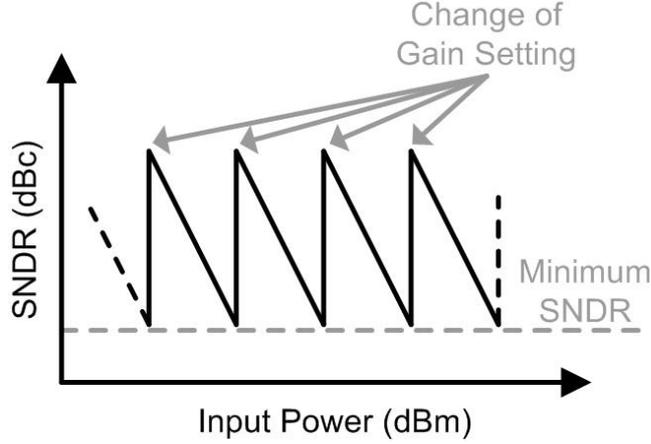
**Figure 2.5:** SNDR vs input power with constant SNDR steps.
