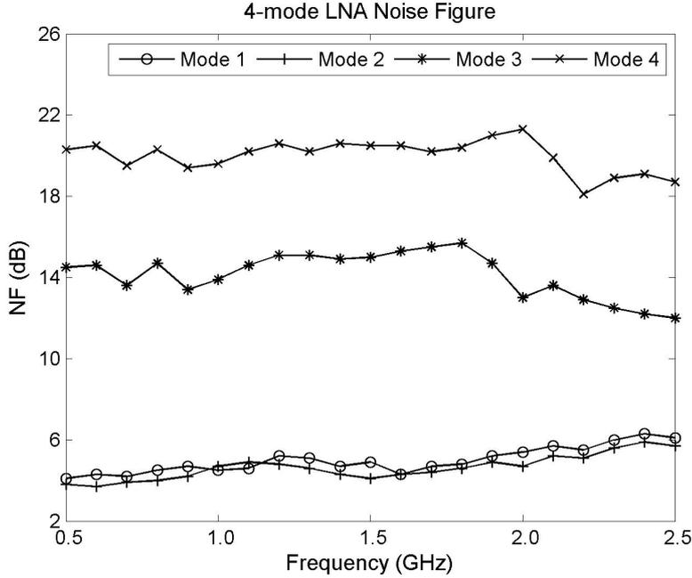
**Figure 4.18:** Measured noise figure of the RFPGA four settings.
