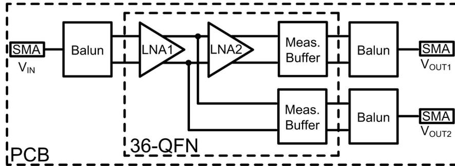
Figure 4.13: PCB measurement setup.
