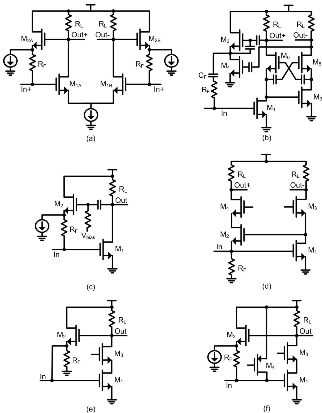
**Figure 3.10:** Alternative active feedback input impedance matching topologies (a) Differential (b) Single-ended to differential conversion with single-branch active feedback (c) AC coupling at the output (d) Single-ended to differential conversion with local feedback (e) Without current source at the feedback (f) Current sink at the input.
