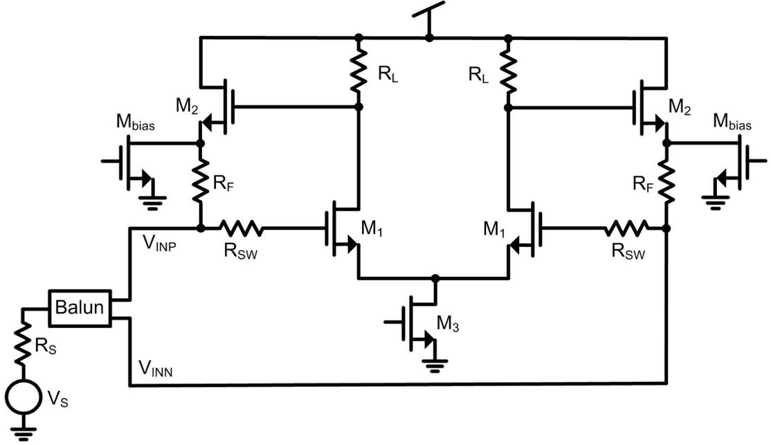
**Figure 4.7:** LNA1 simplified schematic used for noise optimization calculations.
