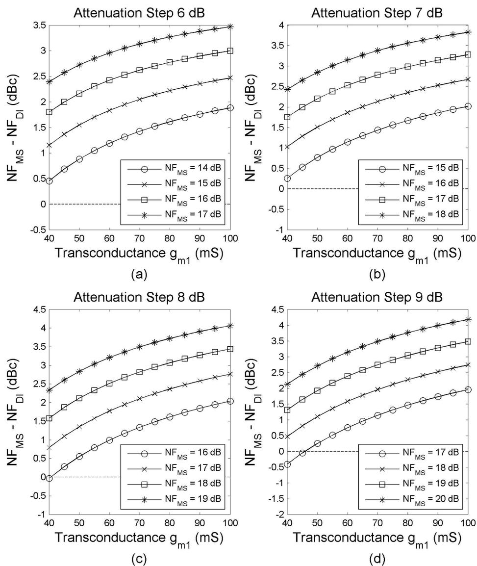
**Figure 5.10:** Noise figure difference between the MS and the DI topologies (Gain Setting 3) for different values of transconductance, MS noise figure and attenuation step.
