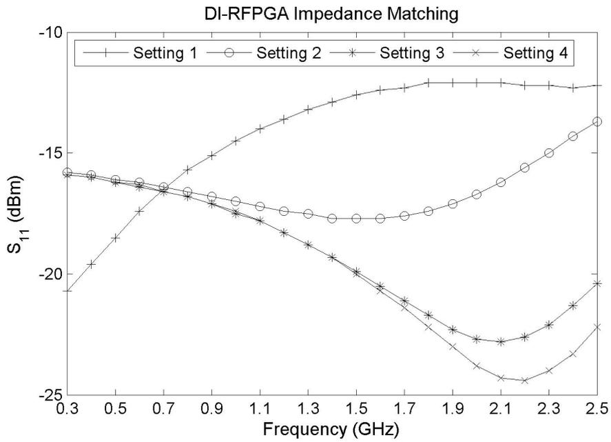
Figure 5.13: DI-RFPGA  $s_{11}$  measurement results.
