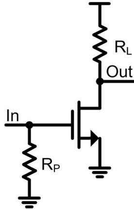
**Figure 3.1:** Basic topology of the parallel resistance input impedance matching.
