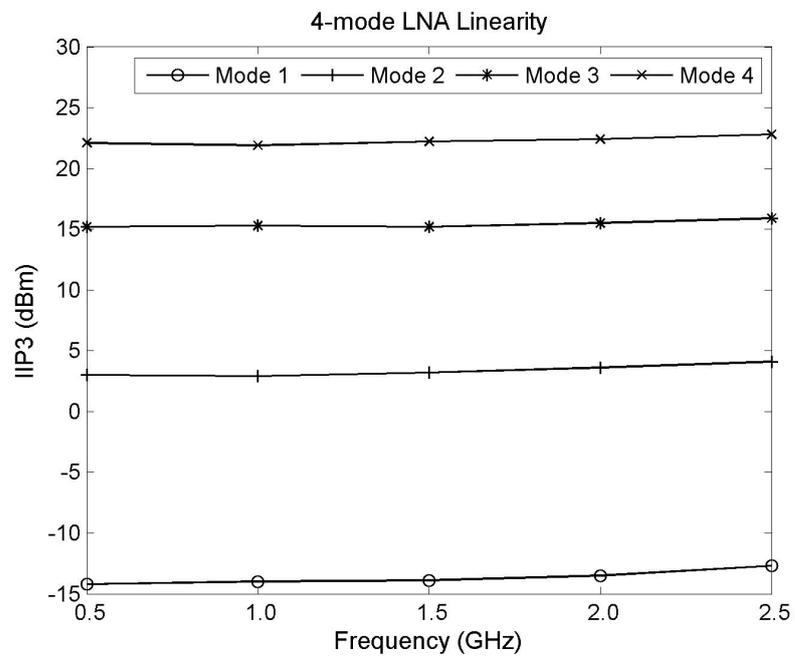
Figure 4.17: Measured IIP3 of the RFPGA four settings.
