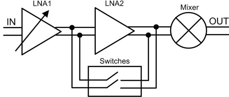
**Figure 4.3:** Proposed configuration of RFPGA prototype I in a front-end implementation.
