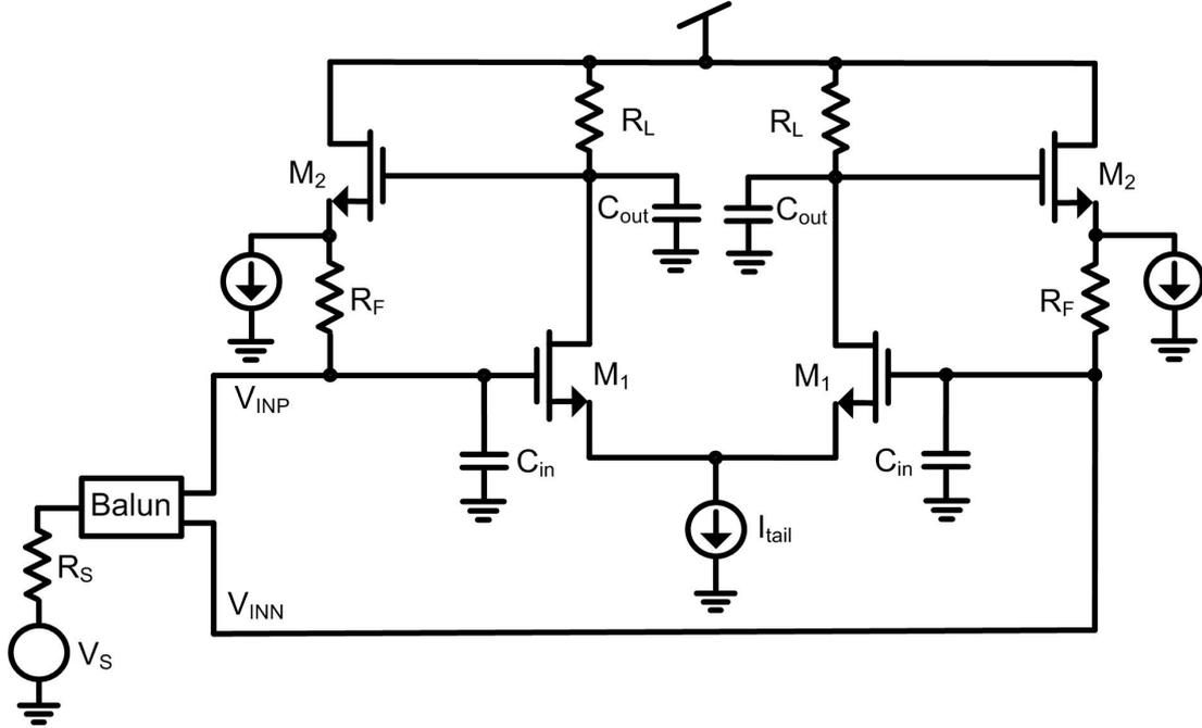
**Figure 4.9:** LNA1 simplified schematic used for input impedance optimization calculations.
