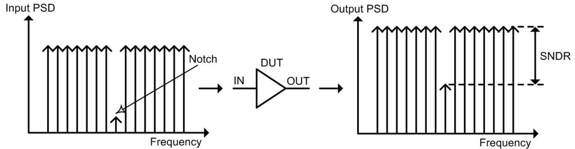
**Figure 2.6:** NPR measurement process.
