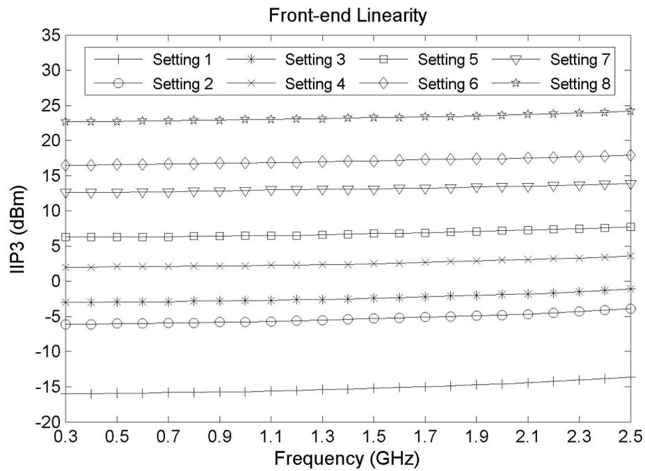
Figure 6.11: Front-end IIP3 measurement results.
