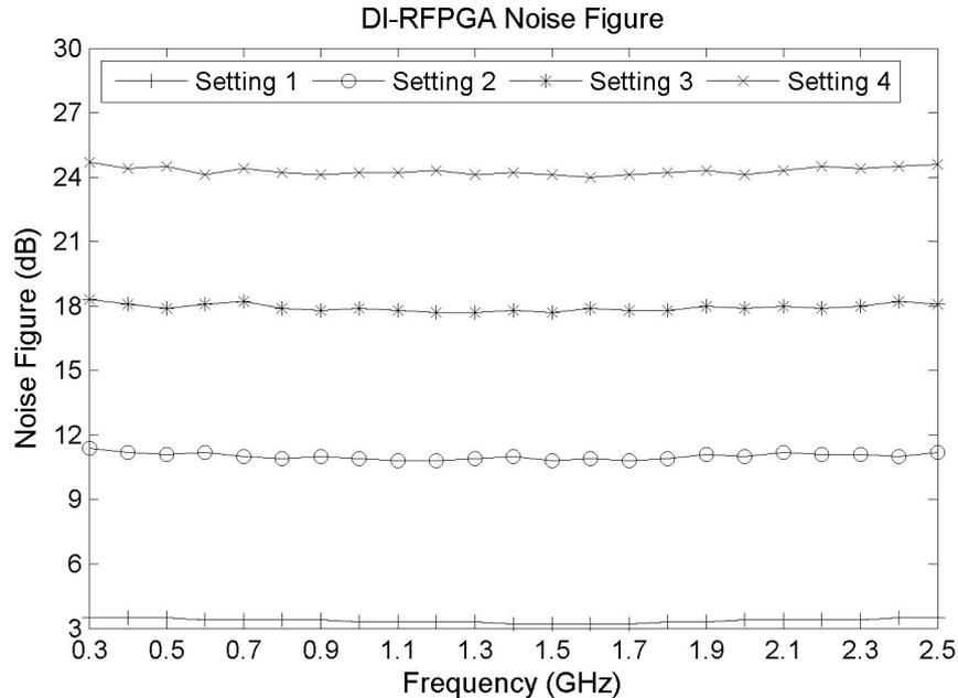
Figure 5.15: DI-RFPGA noise figure measurement results.
