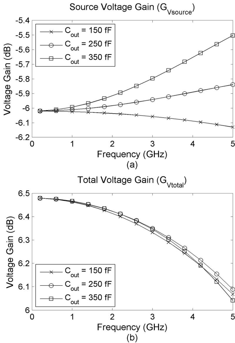
**Figure 4.12:** Voltage gain using the active feedback input impedance matching topology for different values of output capacitance (a) Source voltage gain (b) Total voltage gain (source plus amplifier).
