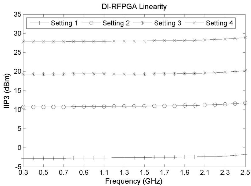
Figure 5.14: DI-RFPGA IIP3 measurement results.
