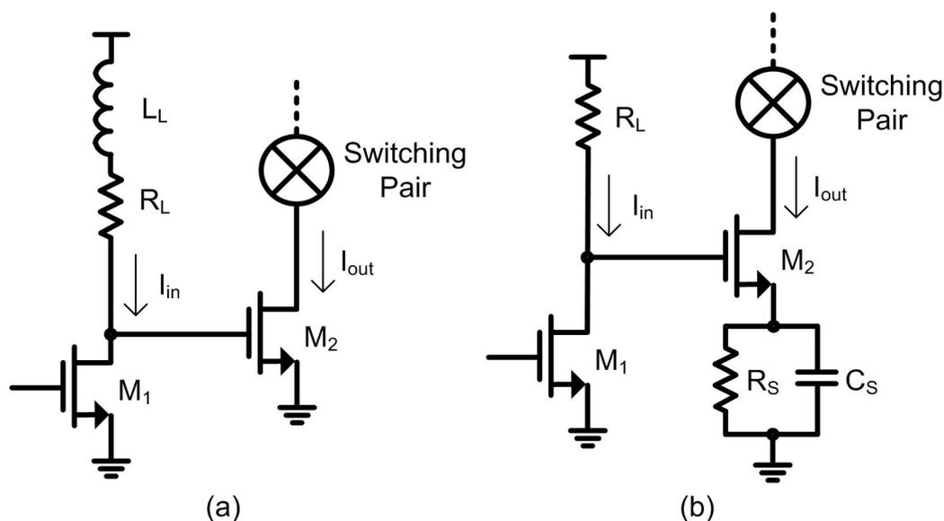
**Figure 3.16:** Techniques for adding a zero in the gain transfer function (a) Inductive peaking (b) Capacitive peaking.
