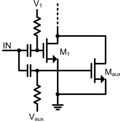
Figure 3.17: Derivative superposition structure.
