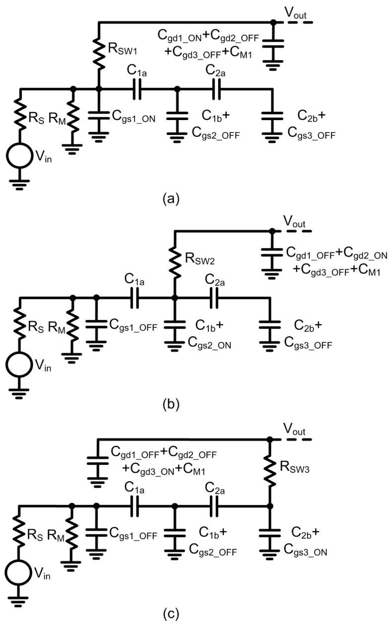
**Figure 4.6:** Circuit model of the capacitor ladder including switch parasitic capacitances and channel resistance for (a) Gain setting 2 (b) Gain setting 3 (c) Gain Setting 4.
