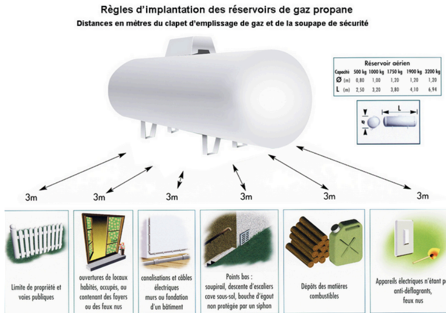
Figure 20. Security distances in aerial tanks [13]
