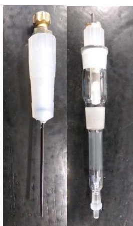
Figure 13. Carbon auxiliary electrode and \text{Ag}/\text{AgCl}/\text{KNO}_3 reference electrode used in the experiments.
