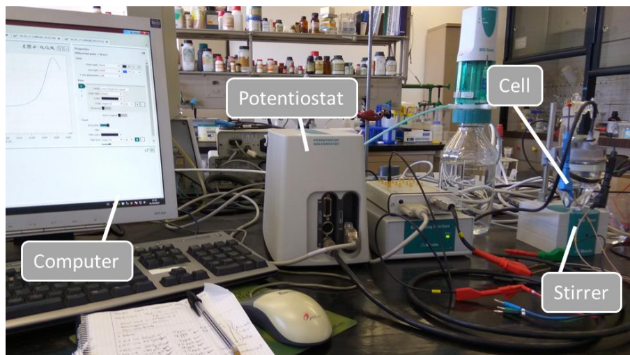
Figure 15. Experimental setup for voltammetric measurements.
