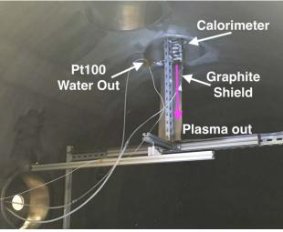
Fig. 5 Calorimeter installation
