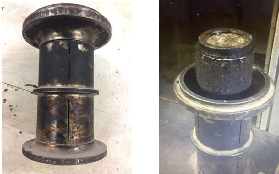
Fig. 2. Slotted moulds used for compacting mixtures.
