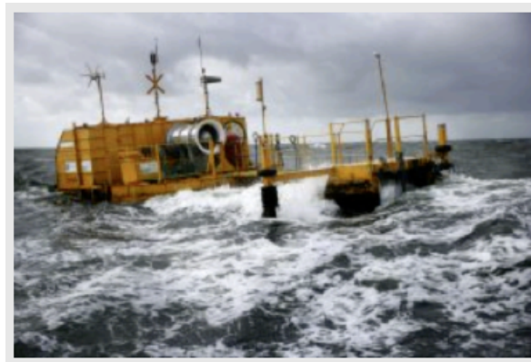
Figure 1.2: Picture of a floating Oscillating Water Column (OWC) device for the extraction of mechanical energy from sea waves. Installation by Ocean Energy [7].
