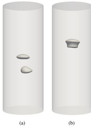
Figure 1.6: Simulation of the merging process between rising bubbles, carried out with Adaptive Mesh refinement techniques. Details in Sec. 3.3.2
