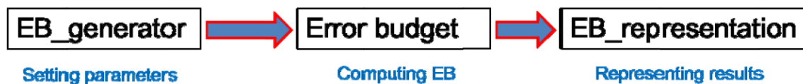
Figure 8.5 Flow graph of the MATLAB program used to compute the Error Budget for the X-MIRAS configuration
