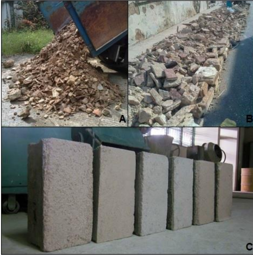
Fig. 1. Source of CDW 1 and 2 (figures A and B, respectively), and recycled mortars placed over concrete blocks (figure C).
