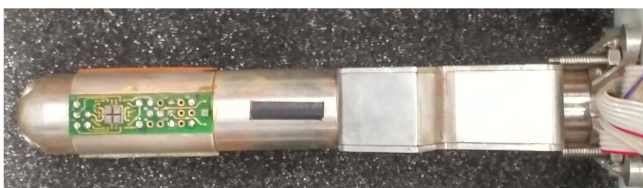
Figure 1: Photography of the proof of concept prototype of REMS wind sensor. One of the PCBs with a group of dice can be seen.
