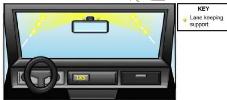
Fig. 9. Smart vehicle actuators (lane keeping support system)
