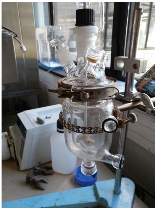
Figure 1.3. Reactor with thermal Shell and paddle stirrer
