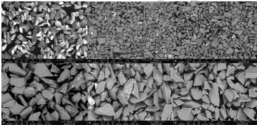
Figure 3.5. Surface SEM images of the SiC coated with Fe 3 O 4 nanoparticles: (a) SiC blank; (b) Procedure 1; (c) Procedure 2; (d) Procedure 3; (e) Procedure 4.1; (f) Procedure 4.3
