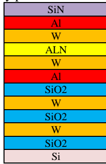
Fig. 3. Stack configuration of the measured SMR BAW resonator.
