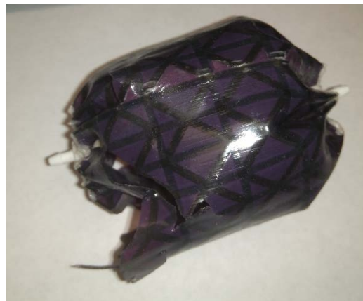
Fig. 51 Actuator broken during the thermomechanical activation process.
