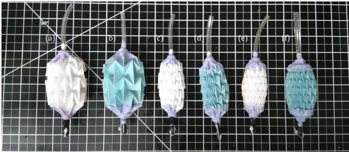
Fig. 22 6 different waterbomb-based prototype actuators: (a) 4x8 in paper, (b) 4x8 in cardboard, (c) 6x12 in paper, (d) 6x12 in cardboard, (e) 8x16 in paper and (f) 8x16 in cardboard.
