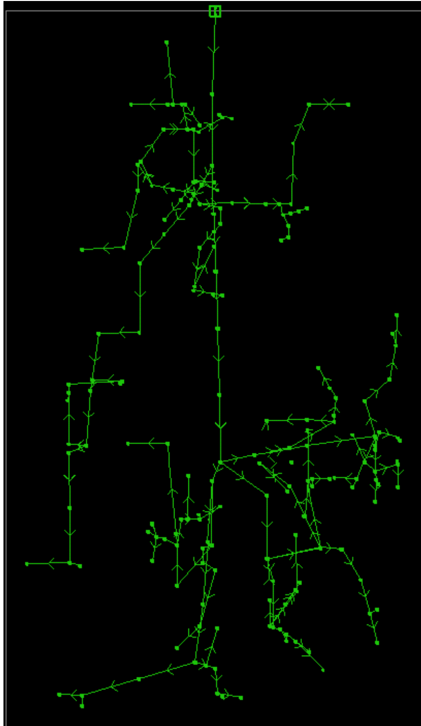
Figure 4.3: Clock tree trunk of Block 2 using the reference clock tree input pin with CCD algorithm.
