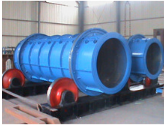
Figure 55. Centrifuge concrete casting machine: turning device and mold engineered by oceana Pre-cast machinery Source: http://concretepipemachine.sell.everychina.com/
