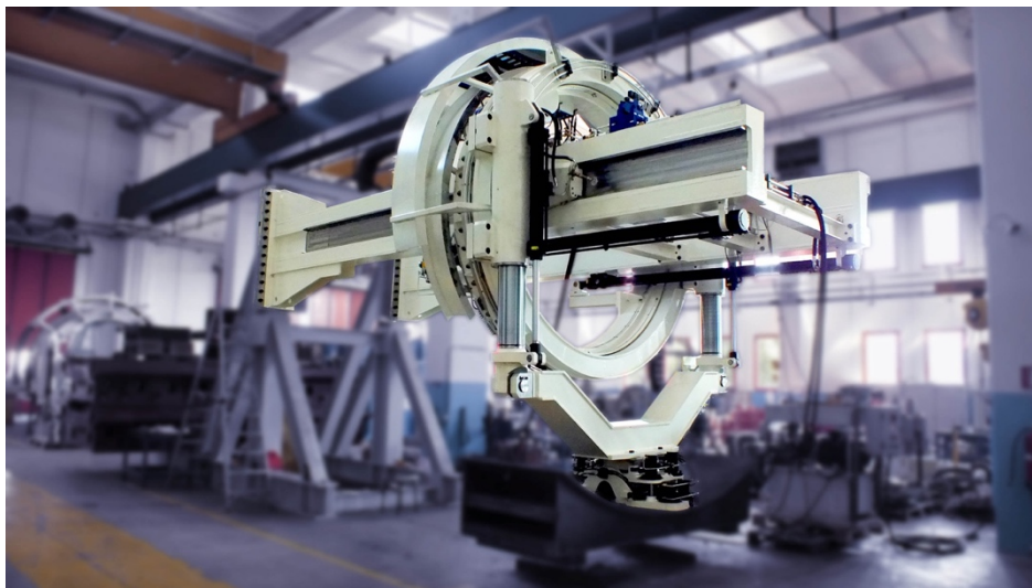
Figure 105. Erector arm designed and built by Galbiati Group, firm specialized on mechanical machines for Engineering and Construction. (Galbiati Group, 2014)
