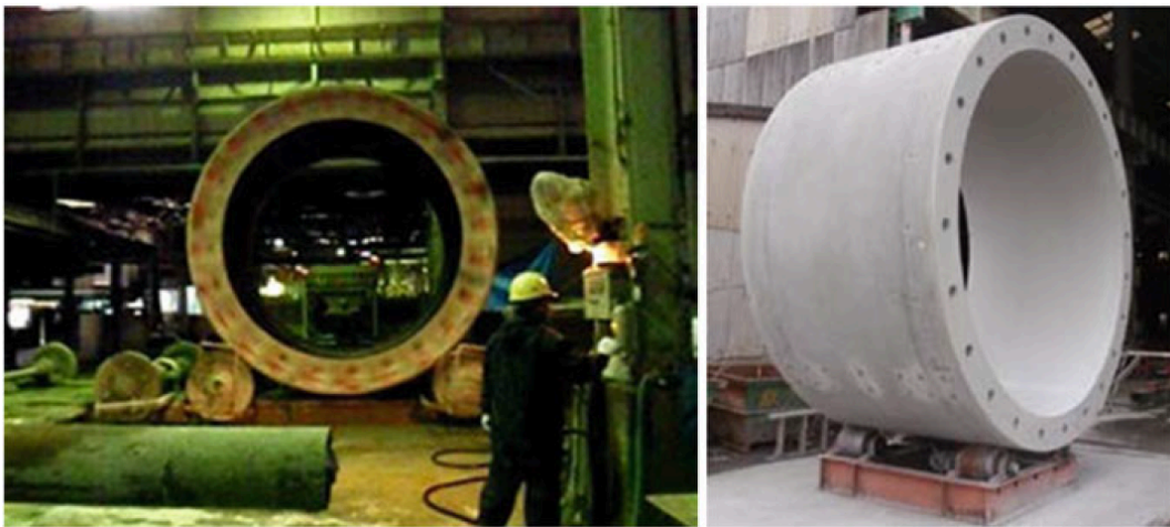
Figure 42. Manufacturing of the centrifugal PC precast segments by centrifugation. Source: (Utsunomiya, et al., 2015)
