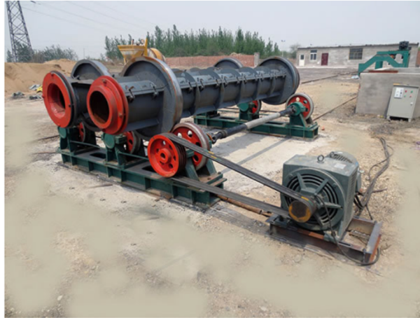
Figure 115. Spinning mechanism using a V-belt.
