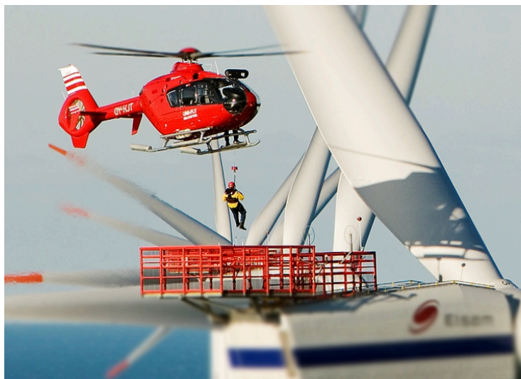
Figure 10. Lowering of personnel on turbine at Horn Rev 1. Source: http://www.uni-fly.dk
