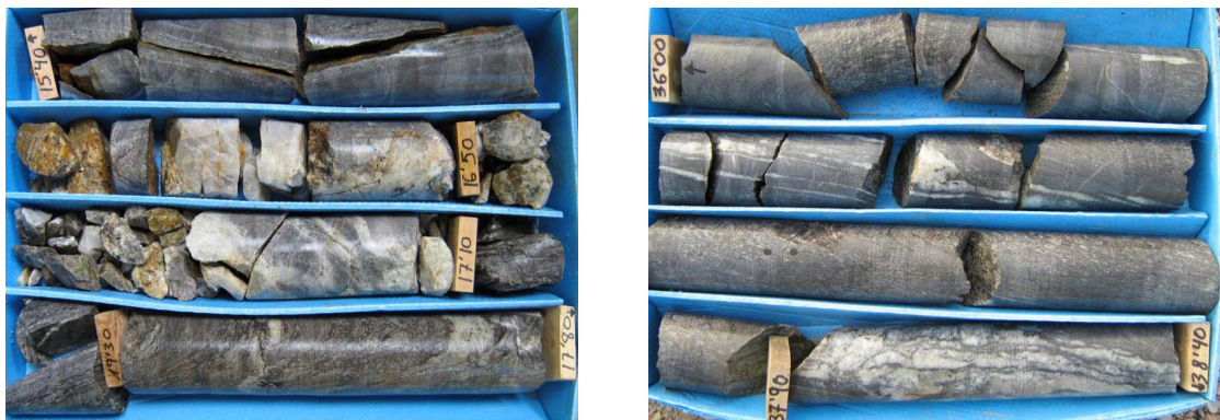
FIGURE 4.9: Left: Outcrop from the borehole S2001, interval from 15.4 to 17.8 meters depth, showing the plausibility of the double behavior assumption. Right: interval from 36 to 38.4 meters depth showing that the rock mass is preferentially fractured horizontally and that the anomalous behavior should come from a discrepancy between the transmissivities of each fracture.
