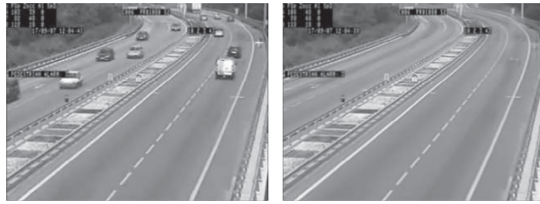
Figure 5.1: Adaptive background learning after 750 iterations with \alpha = 0.01 . The left image is the input video and the right one is the background model obtained.
