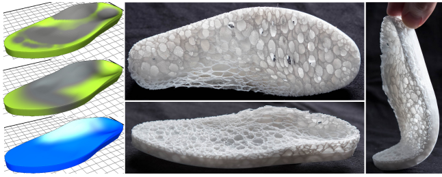
Fig. 24. A 3D printed shoe sole. Left : Control fields used on the model, density (top), orthotropy strength (middle) and angle (bottom). Right : Printed shoe, top, side and bending. The shoe is printed without any skin to reveal the foam structure.
