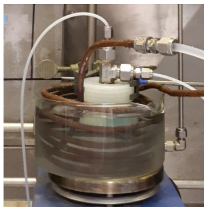
Figure 40 Small-scale fluorination set-up using F_2/N_2 (10% v.v -1 )
