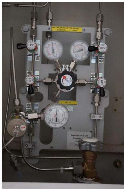
Figure 11 Pressure-controlled system between the commercially available F_2/N_2 (20% v.v -1 ) and smaller storage cylinders connected to reactive batch glass systems
