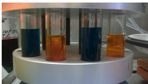
Figure 33 Picture of reaction mixtures containing 2-fluoro-1,3-dimethylmalonate, olefin and Mn(OAc)_3 with and without Cu(OAc)_2 as co-catalyst
