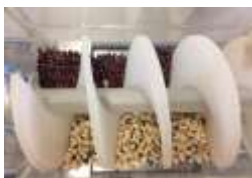
Fig. 3: Placing the material (mung beans and black eye beans) in the variable speed screw blender
