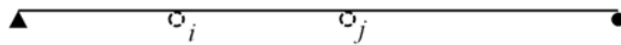
(a) Simply supported beam with an assumed “perturbed” boundary condition with added pins at “i” and “j”
