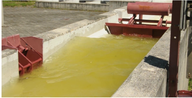
Fig. 1. Photo of an experimental AMIL gate exhibiting oscillating behaviour and creating waves.
