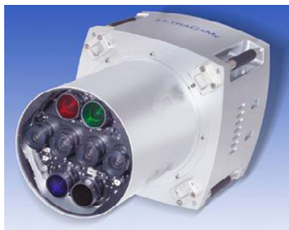
Figure 93. Vexcel's Ultracam XP camera. (Source: Vexcel Corporation)
