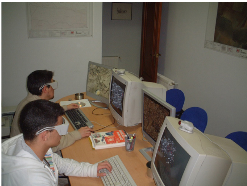
Figure 54. Stereoscopy by temporal separation.
