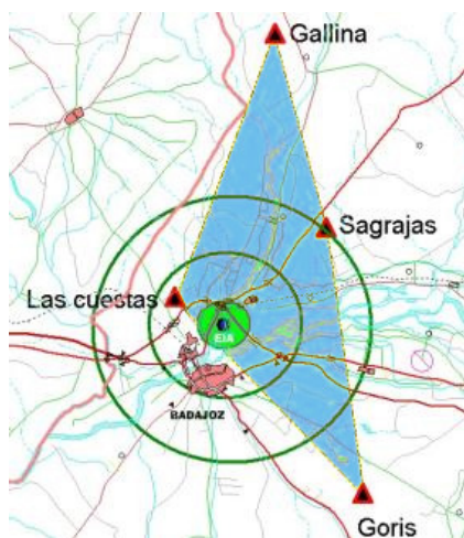
Figure 26. Example of how data is gathered for the WGS84-ED50 transformation.
