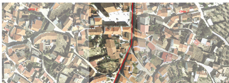
Figure 146. Correct union delimitation between orthophotos.
