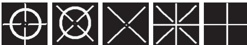
Figure 102. Standard patterns for fiducial marks.
