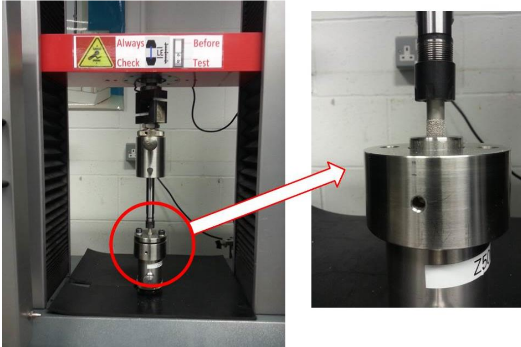
Figure 4 Picture of the insertion and removal test arrangement on the Zwick Z-50.
