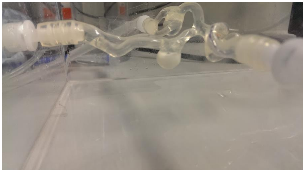
Figure 5.4.12 Hydrogel injected in to the aneurysm model with physiological flow applied
