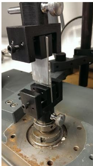
Figure 4.6.3 Bond strength test set-up
