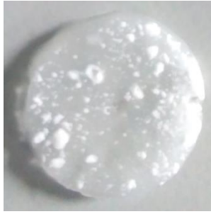
Figure 5.7.5 Bioactive glass - Alginate hydrogel after Von Kossa staining
