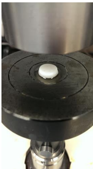
Figure 4.6.1 Hydrogel sample following compression testing
