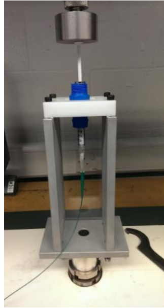
Figure 4.6.4 Testing the force required to inject the hydrogel through a microcatheter
