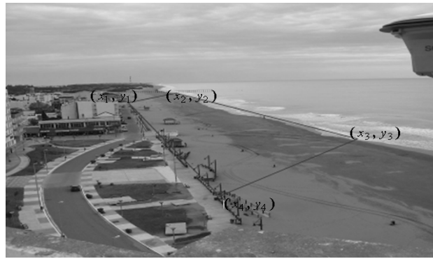
Fig. 2. Control Points ((x_1, y_1), (x_2, y_2), (x_3, y_3), (x_4, y_4)) whose geographic coordinates were obtained with a Global Positioning System and are related with the pixels coordinates in the image.
