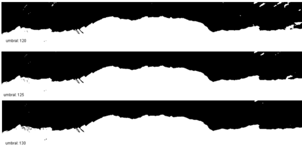
Fig. 7. Images binarized with different threshold values. Empirically, the middle one performs best in the further processing steps.
