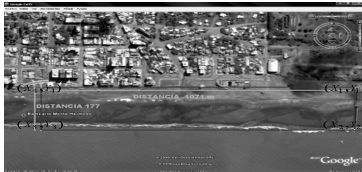
Fig. 3. GPS-established control points taken in the image. These geographic coordinates determine the parameter of the projection matrix.
