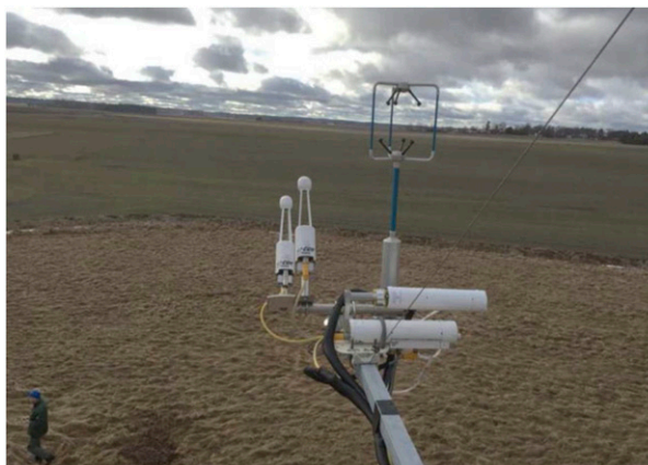
FIG. 1. A picture of the instrument setup with four Li-Cor instruments and the Gill sonic anemometer at the field measurement site Marsta near Uppsala.
