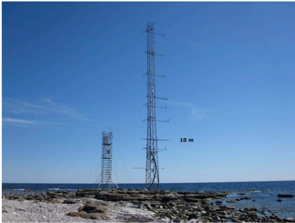
FIG. 2. A picture of the 30-m tower at the Östergarnsholm site with the 10-m level indicated. Also seen is a smaller tower instrumented for measurements of marine aerosols.
