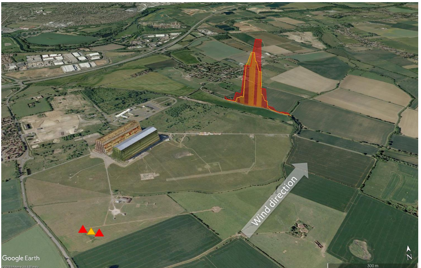
Figure E4.11 Release 11 gas release points, wind direction and monitoring route. Transect DTU 11.3 (Google Earth 2017)
