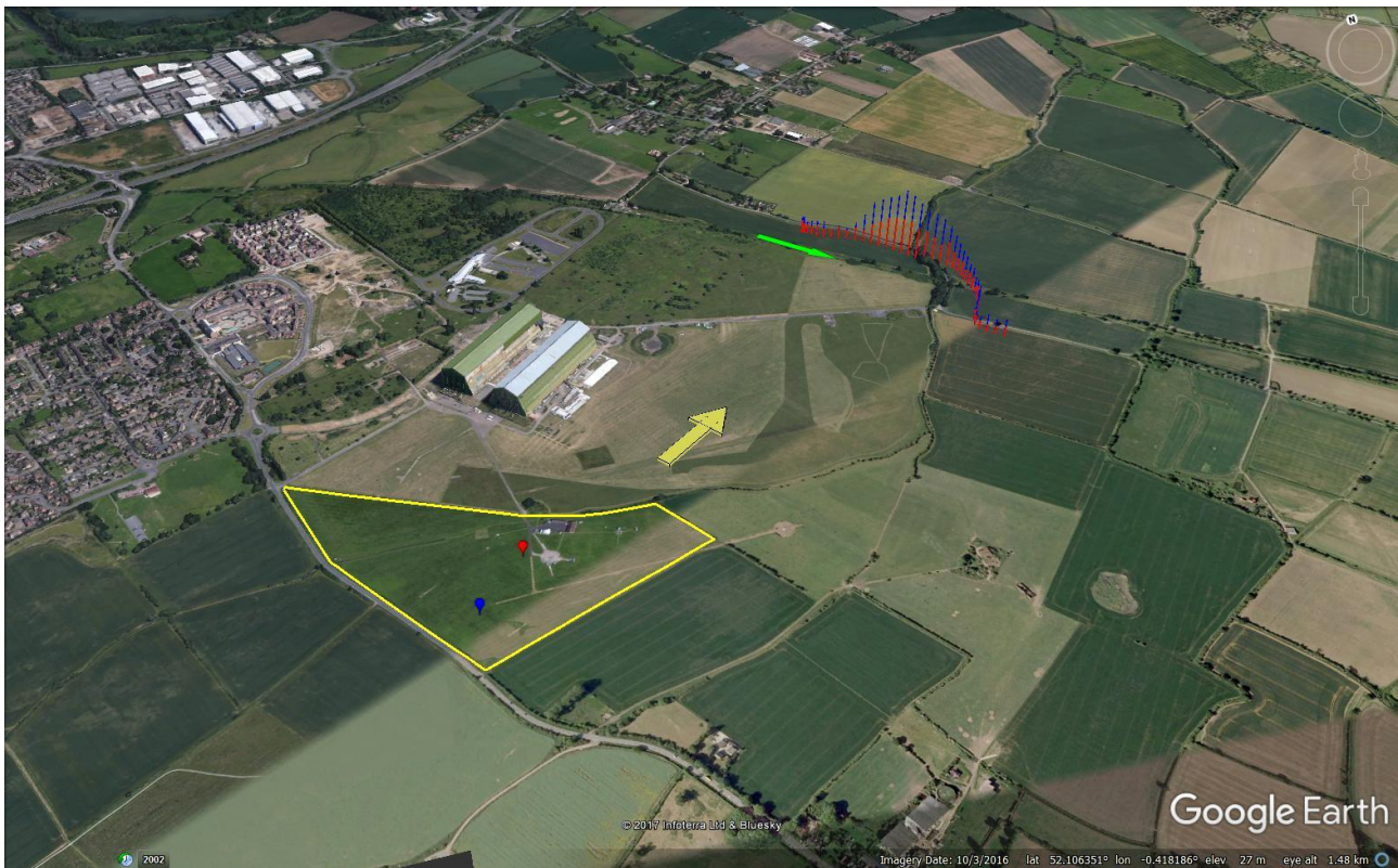
Figure E4.4 Release 9 gas release points, wind direction and monitoring route. Transect UOS 9.6 (Google Earth 2017)
