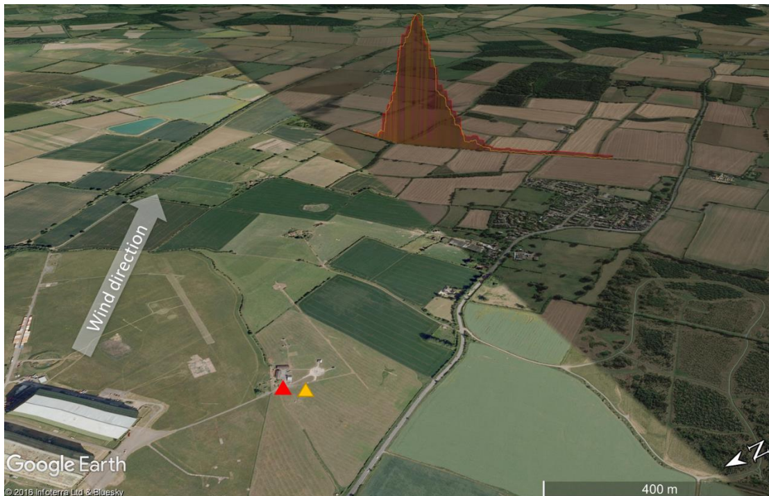
Figure E4.8 Release 8 gas release points, wind direction and monitoring route. Transect DTU 8.25 (Google Earth 2017)
