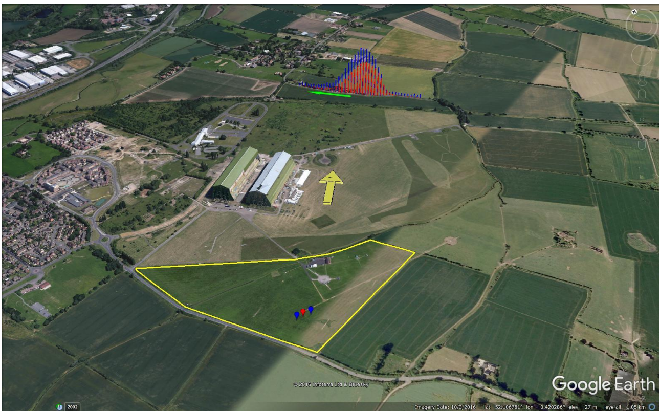
Figure E4.6 Release 11 gas release points, wind direction and monitoring route. Transect UOS 11.7 (Google Earth 2017)
