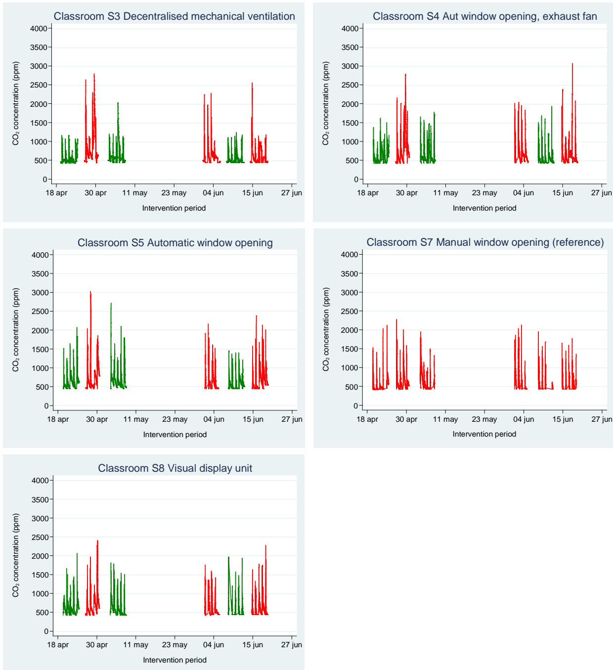
Figure 6.3.2. Weekly profiles of the CO 2 concentration measured in each classroom during the six-week intervention period in the non-heating season. Red: System control idled, Green: System control activated.
