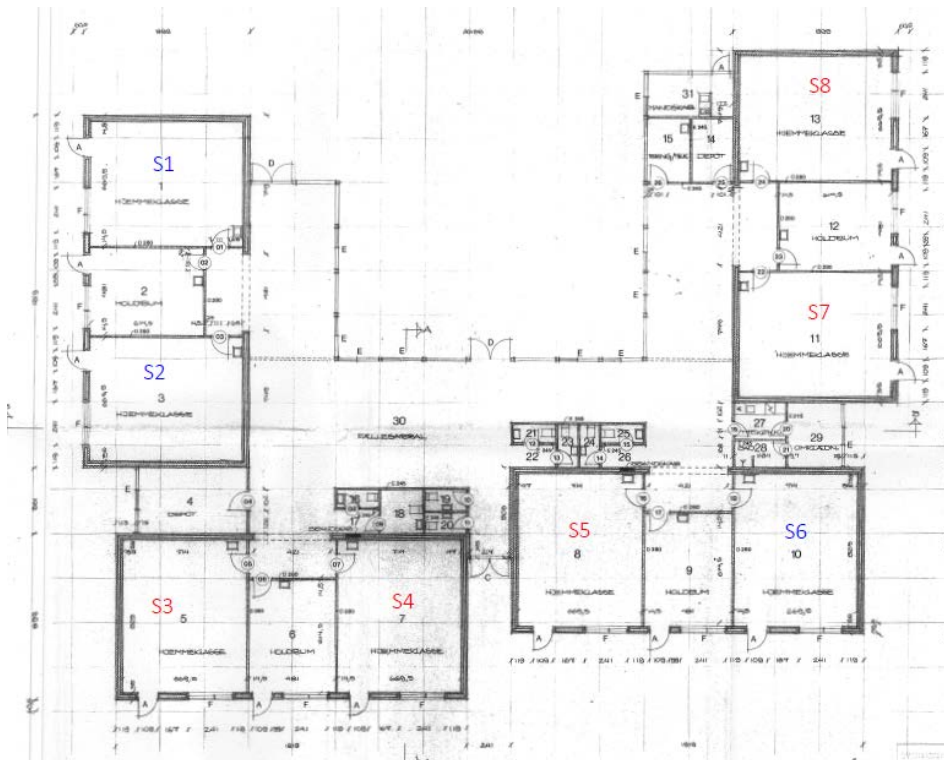
Figure 5.1.3. Plan drawing of the south wing where the intervention studies took place. Numbers in red indicate the classrooms that were included in the study. A decentralized mechanical ventilation system was installed in classroom S3. A system with automatic window opening assisted by an exhaust fan was installed in classroom S4. A system with automatic window opening and heat recovery units was installed in classroom S5. No special systems were retrofitted in classrooms S7 and S8. Pupils in classrooms S8 used a device that provided visual feedback on the CO 2 concentration indicating when the windows should be opened.
