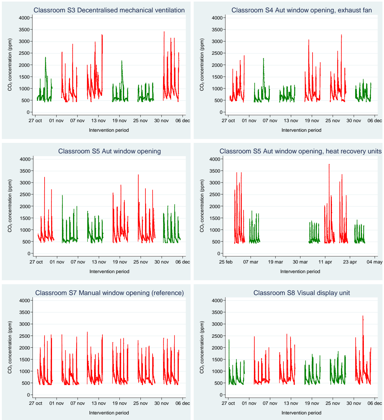
Figure 6.3.1. Weekly profiles of the CO 2 concentration measured in each classroom during the six-week intervention period in the heating season. Red: System idled, Green: System activated.
