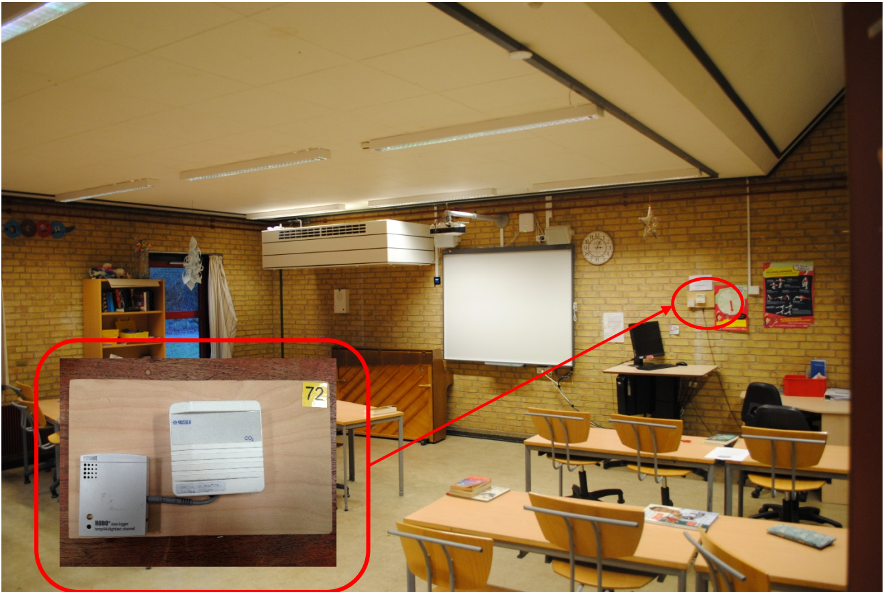
Figure 5.1.12. Measurement station with a CO 2 transmitter and a datalogger that also recorded temperature and air humidity.
