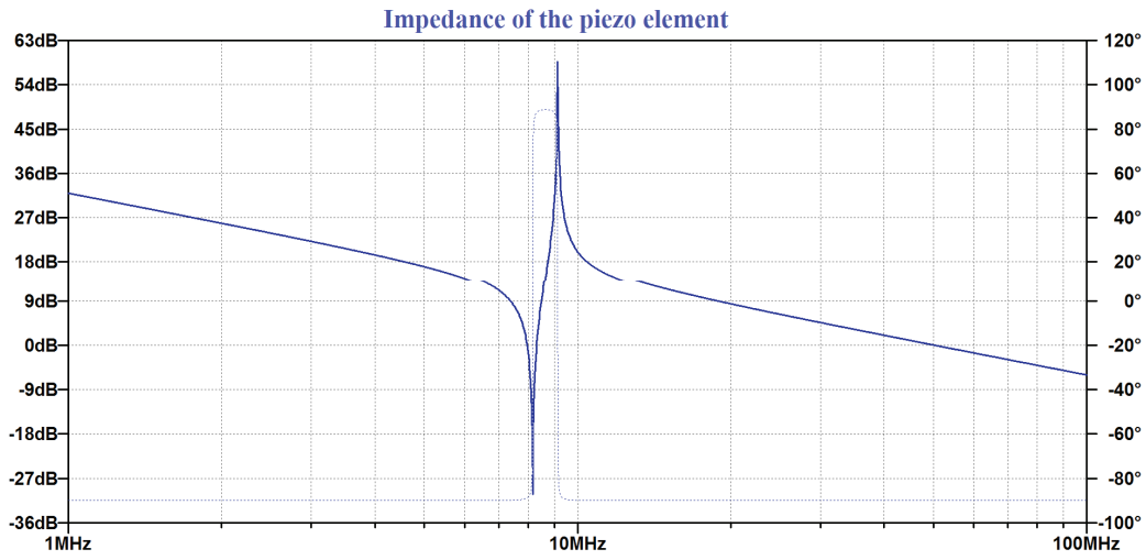
Fig. 4.16 Simulated impedance of the piezo element in Table 4.3.
