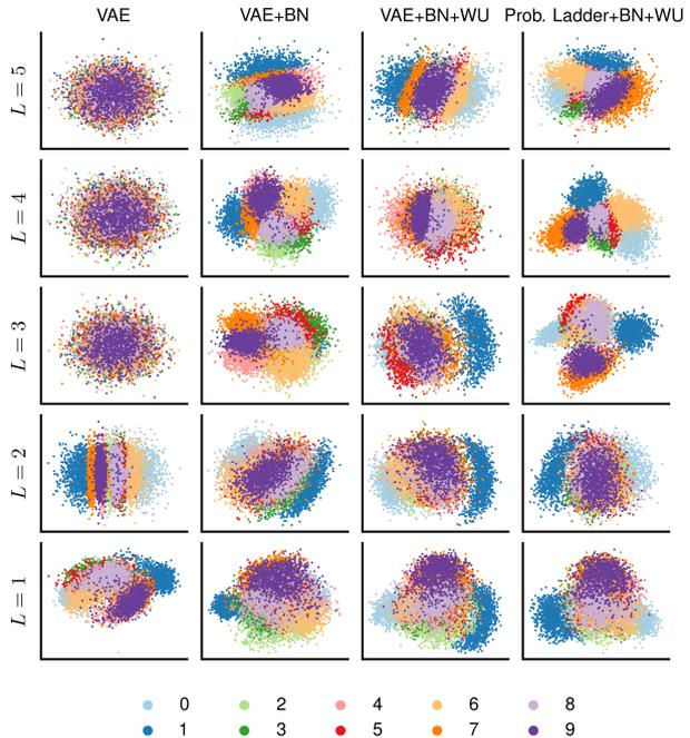
Figure 7. PCA-plots of samples from  $q(z_i|z_{i-1})$  for five layer VAE and probabilistic ladder networks trained on MNIST. In the vanilla VAE the stochastic units above the second layer is clearly seen to be inactive with no dependency on the the input data. For the other models a clear structure according to class is seen for the higher layers.
