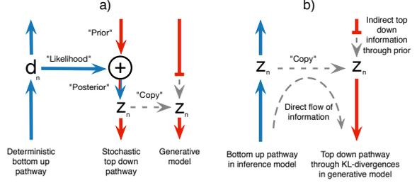
Figure 2. Flow of information in the inference and generative models of a) probabilistic ladder network and b) VAE. The probabilistic ladder network allows direct integration (+ in figure, see Eq. (21)) of bottom-up and top-down information in the inference model. In the VAE the top-down information is incorporated indirectly through the conditional priors in the generative model.
