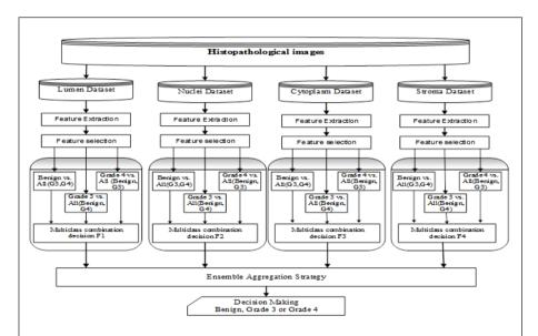
*Figure 4.* The architecture of the Ovall with the ensemble framework (ensemble\_Ovall) for addressing the three-class classification problem in PCa grading.
