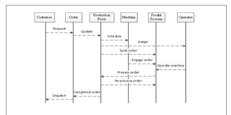
Figure 2. The System Message sequence diagram.
