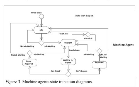
In Figure 3, the machine in the initial state idles when no order is being processed or is waiting. The machine becomes engaged as the order arrives, is being processed, or when orders are waiting in queue the machine continues to be engaged. In the case of machine breakdown, three states can occur: which can be waiting for repair,
