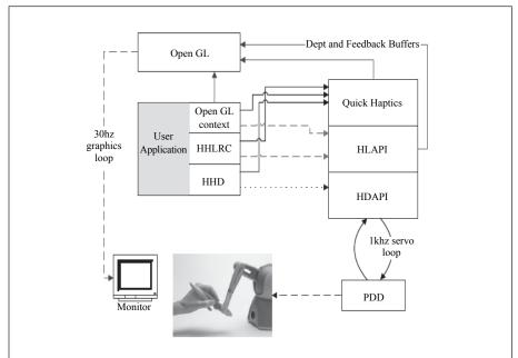
Figure 3. An overview of the OpenHaptic Toolkit (adapted from Sens Able Technologies.)
