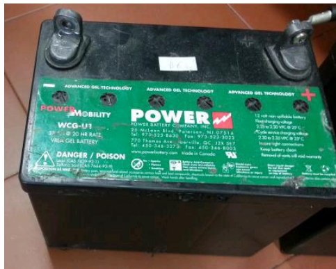
Figure 6.5 - VRLA GEL battery that is used in the project.
