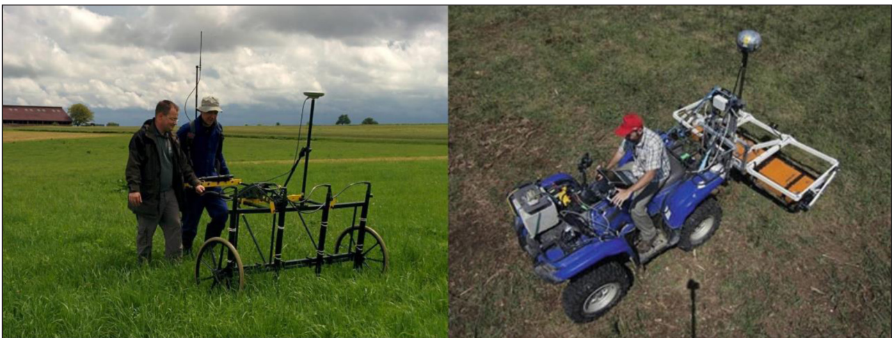
Figure 1: Multi-sensor array geophysics in action. Left: magnetic gradiometry, right: multichannel GPR survey (image courtesy Alenandre Novo and Geostudi Astier).
