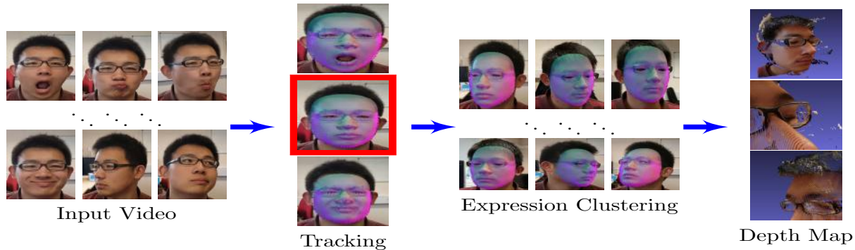
Figure 1: Given a video, a parametric 3D model [6] was fitted to noisy 2D landmarks produced from the off-the-shelf 2D landmark detector[21]. The fitted 3D model is used to refine the 3D position computed from the 2D landmarks via robust photometric tracking. The tracked 3D mesh are superimposed on the image. After clustering, video frames of similar facial expressions as seen at different viewing angles are used to compute a complete and smooth dense depth map. The glasses and hair are well reconstructed.
