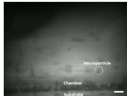
FIG. 6. A video shown a single 20- \mu\text{m} microparticle trapped at a 3D node by switching on the input power. (Multimedia view) [URL:]
