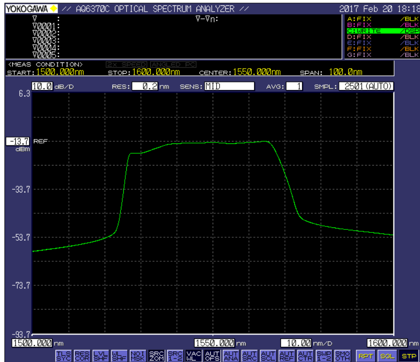
Figure 4.6 The spectrum of the C-Band light source used for this experiment
