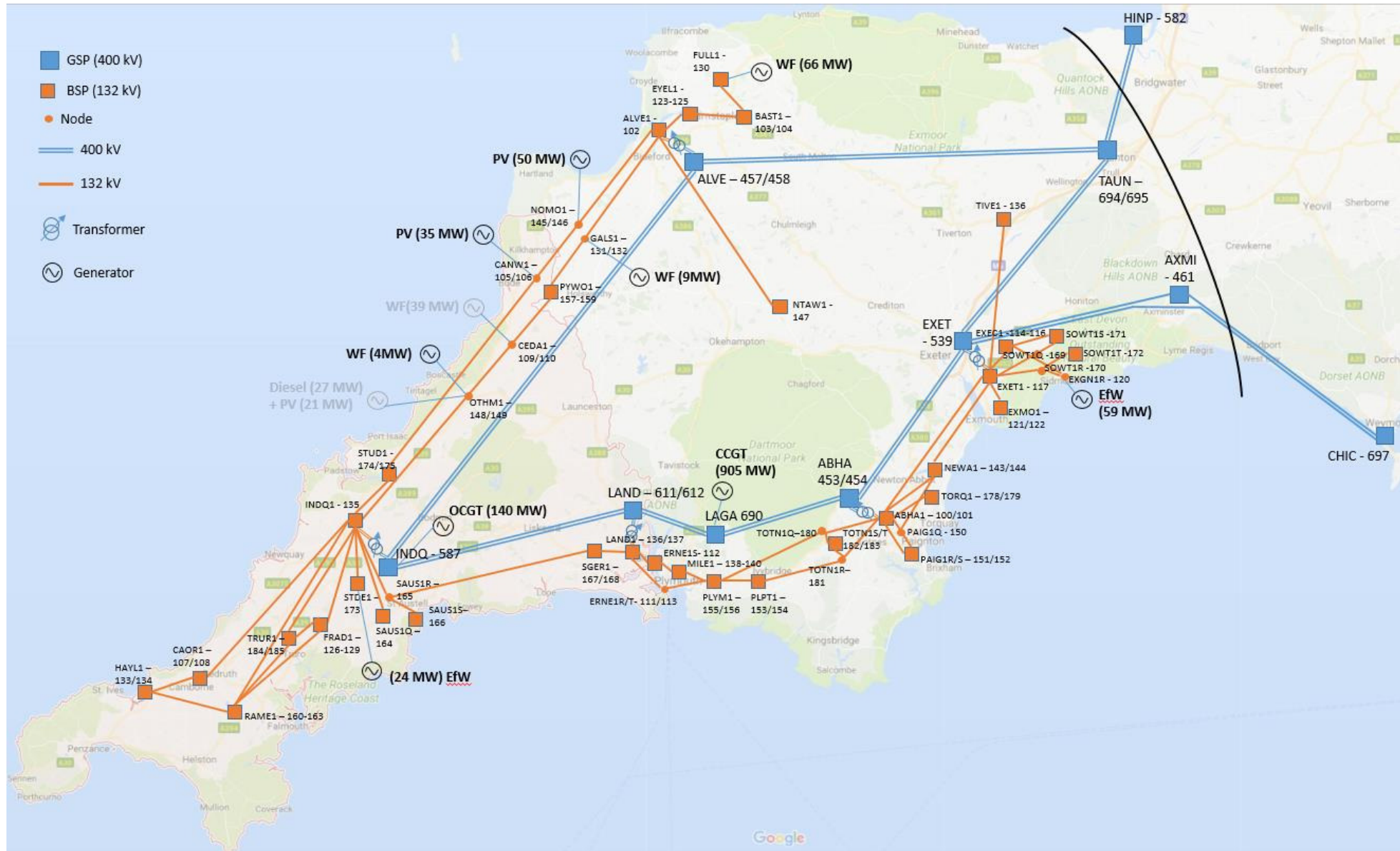
Figure 15 - South West 400kV and 132kV networks with codes from LTDS and numbers used in Matpower modelling
