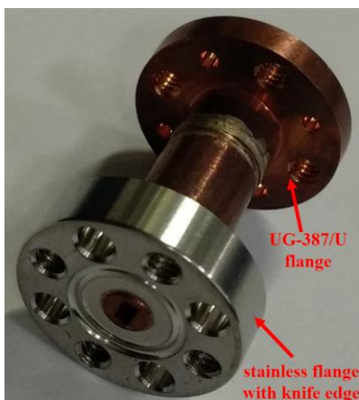
Fig. 4 The pillbox window after brazing assembly.
