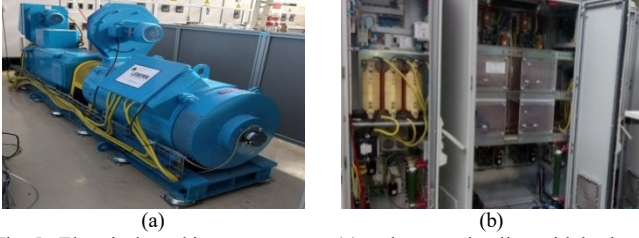
Fig. 5. Electrical machine arrangement (a) and conversion line with back-to-back NPC converter arrangement (b).
