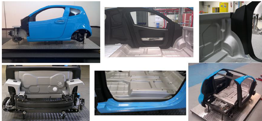
Figure 19 Details of work-in-progress EVolution technological mock-up with integrated demonstrators (see online version for colours)
