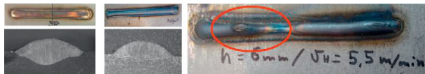
Fig. 8. Beads obtained by TopTIG on AISI 316L. Left) 1 kg/h. Centre) 1.5kg/h. Right) 1.6 kg/h.
