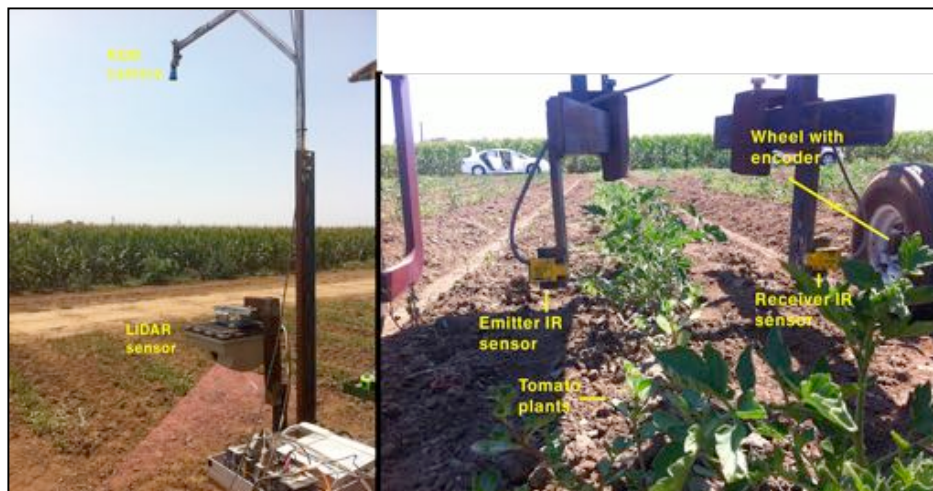
Figure 2. Sensors mounted on the experimental platform designed for field trials in UC Davis, California
