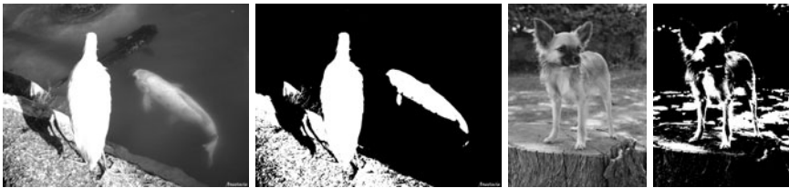
Fig. 3. Binarization using the Hamadani Algorithm. Thresholds are 172 and 155 to each image, respectively.
