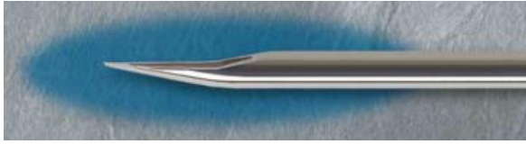
Fig. 2. Detailed picture of the needle point used in the experiments.
