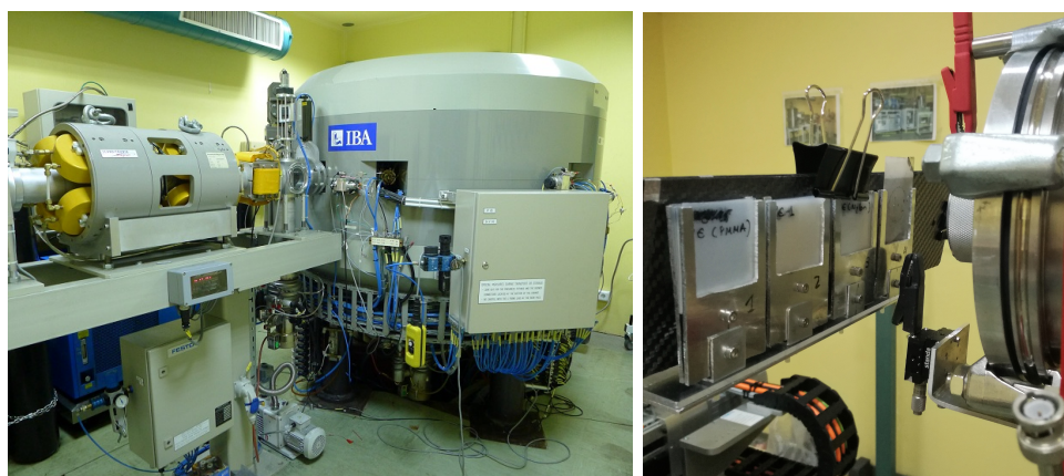
Figure 2.2: Left: 18 MeV (protons)/9 MeV (deuterons) cyclotron accelerator. Right: Experimental set-up, where one can see the sample holders with the different targets inside them, the external beam and the monitored table.
