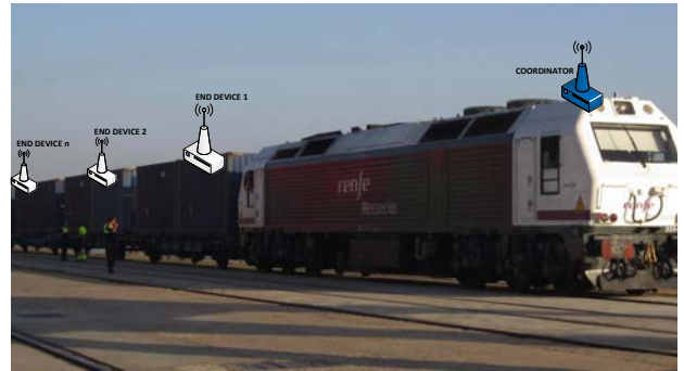
b) Network deployed in a cargo train
