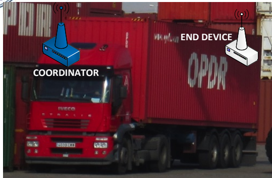
a) Network deployed in a truck: one end device in a container
