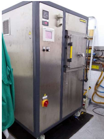
Figure 3.6. High-temperature furnace used for the infiltration and the evaporation processes
