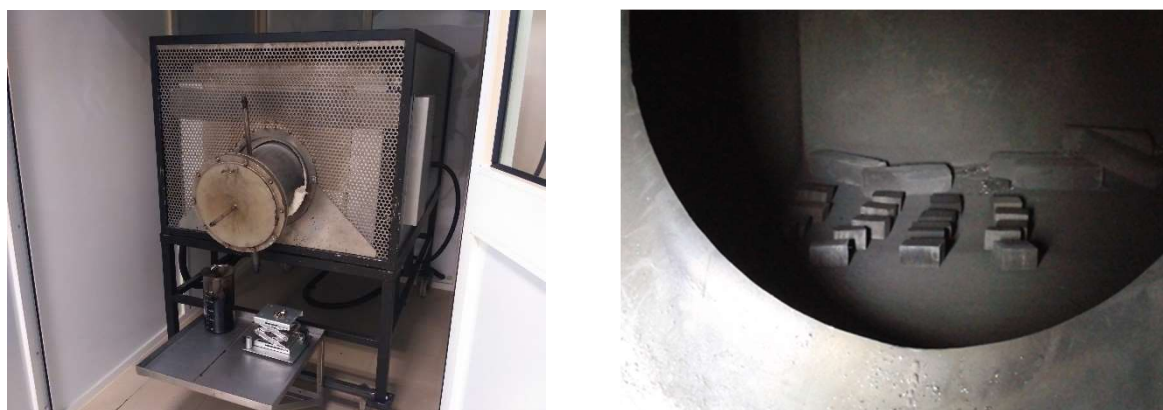
Figure 3.3. Pyrolysis furnace on the left hand side. On the right hand side, inside view of the furnace with the carbon blocks obtained after the pyrolysis
