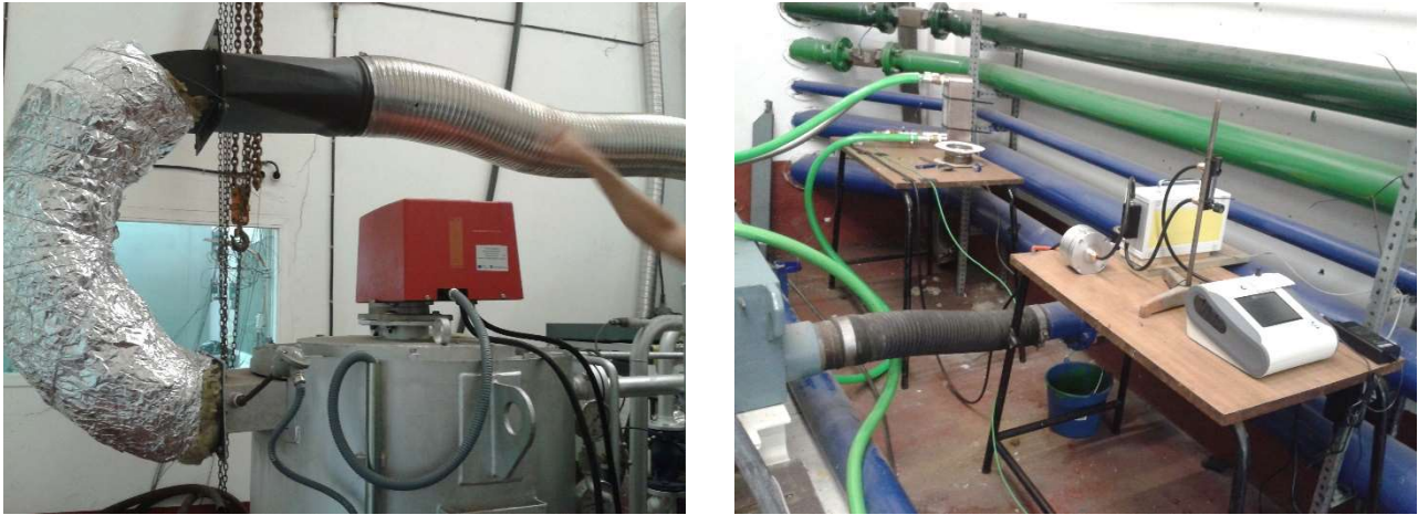
Figure 3.11. Experimental facility for the preliminary measurement of the filtration efficiency: diesel boiler (left) and test rig (right).
