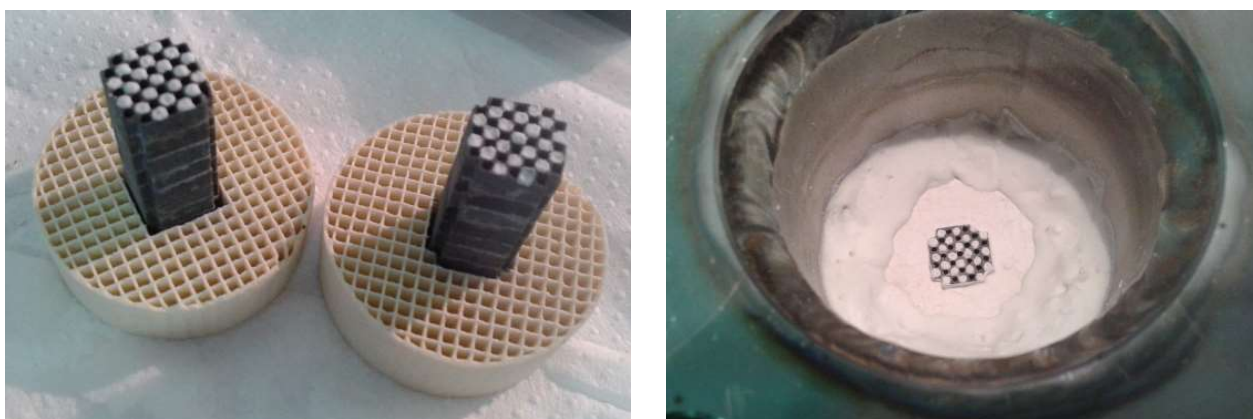
Figure 3.19. Final aspect of the samples in the cordierite adaptor (left) and fitting of the samples inside the canning (right)
