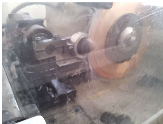
Figure 3.4. Cutting of the carbon cylinders into disks in the precision slicing machine
