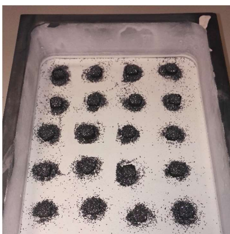
Figure 3.15. Carbon slices of the prototype in the crucible covered with silicon
